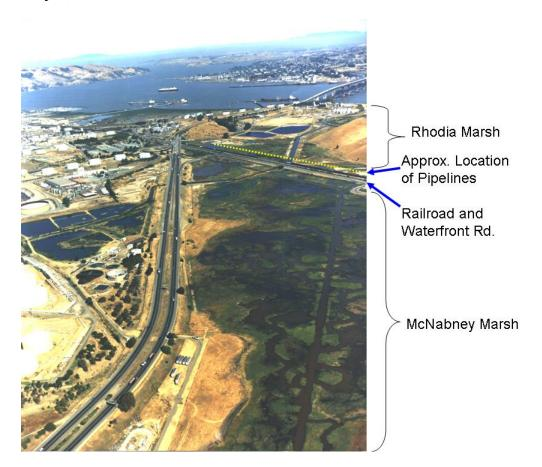
A major obstruction to allowing brackish Bay water to reach McNabney Marsh were four Kinder Morgan pipelines which reduced flow in to (and out of) McNabney Marsh. In October of 2007, Kinder Morgan removed the restriction by lowering the four pipelines. The net benefit is that increased flow will amplify tidal inundation, transforming more of McNabney Marsh from freshwater wetland to salt marsh.
