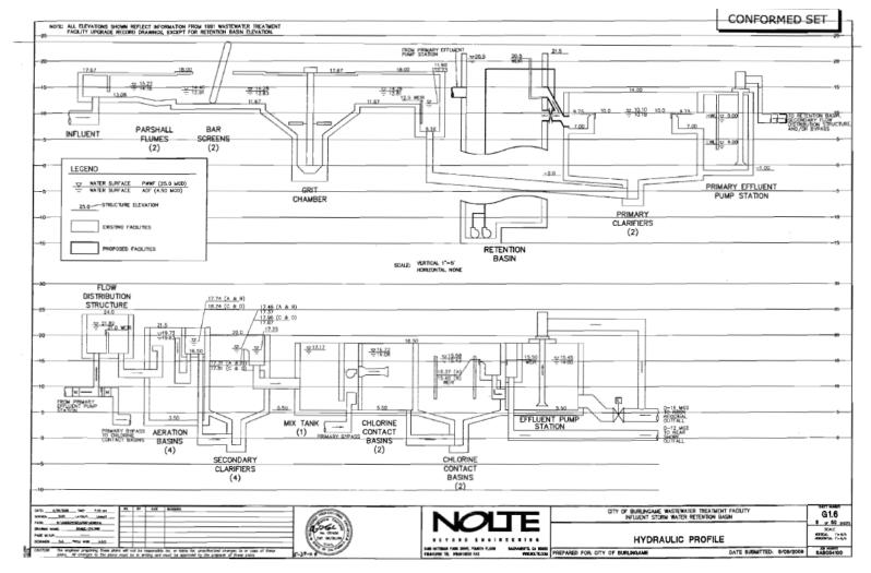
Figure 1. Flow Schematic for the City of Burlingame Wastewater Treatment Facility
