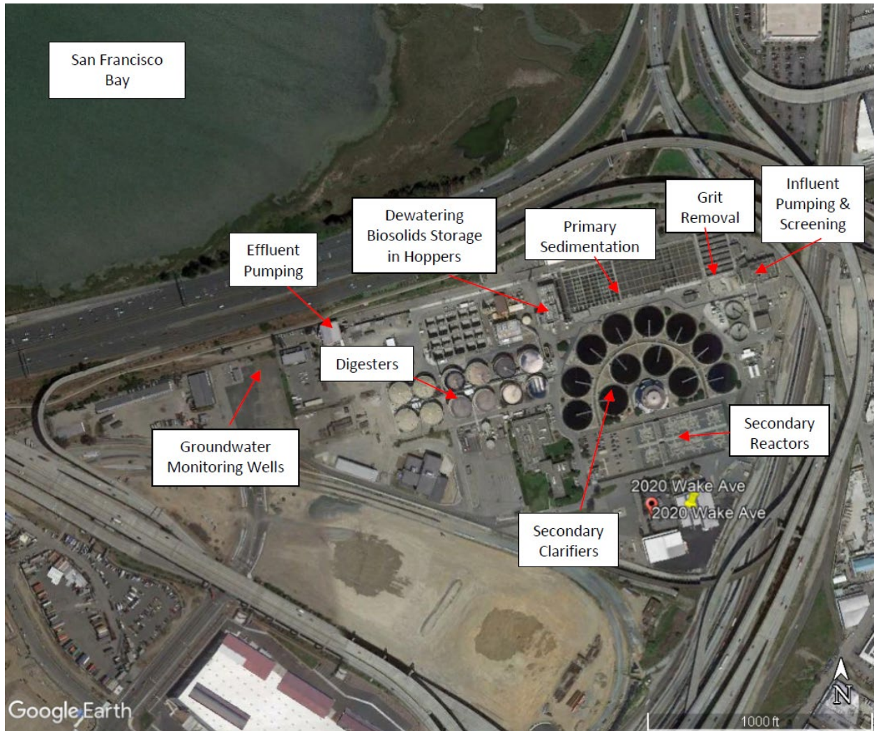
Figure B-2. Topographic / Satellite Map of Major Unit Processes, Wells, and Surface Waters
