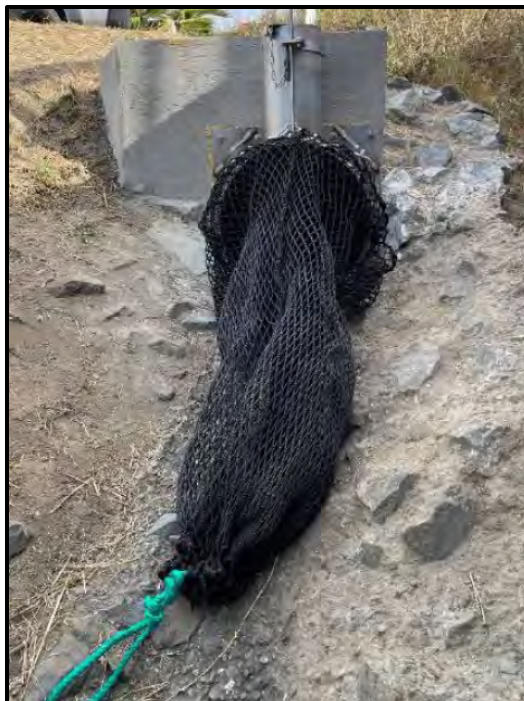
Figure 2: Example of the netting devices used to collect trash during outfall monitoring. This trash net was installed at the Grayson Creek outfall in Contra Costa County. Source: “ Trash Outfall Monitoring Progress Report, Water Year 2024 ,” Watching Our Watersheds Regional Trash Monitoring Project, March 31, 2025.
