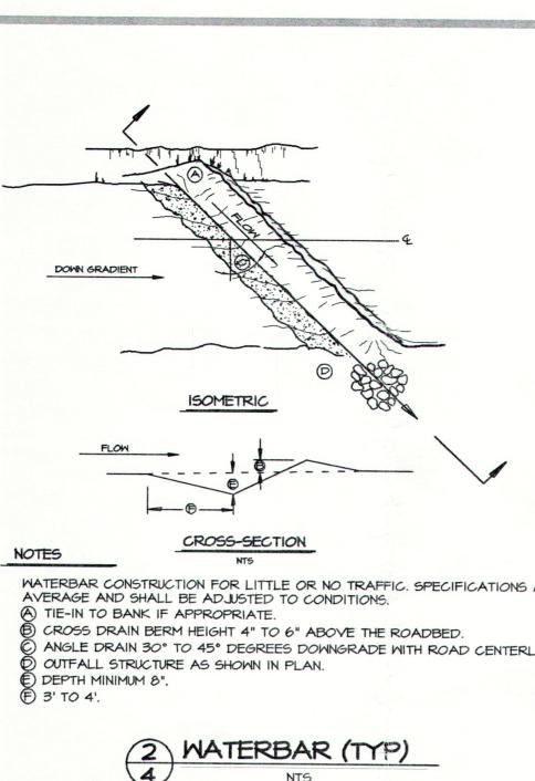
WATERBAR CONSTRUCTION FOR LITTLE OR NO TRAFFIC. SPECIFICATIONS ARE ANGLE DRAIN 30° TO 45° DEGREES DOWNGRADE WITH ROAD CENTERLINE.
