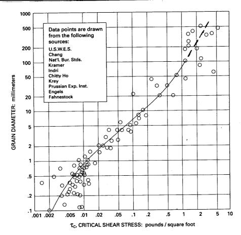
Figure 11.4 Laboratory and field data on critical shear stress required to initiate movement of grains (Leopold, Wolman, and Miller 1964, p. 170). The solid line is the Shields curve of the threshold of motion transposed from the  $\theta$  versus  $R_g$  form into the present form, in which critical shear stress is plotted as a function of grain diameter.
