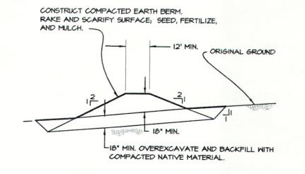
THE TOP OF THE BERM SHALL BE LEVEL, AND SHALL TIE INTO NATIVE GROUND AT EACH END. LENGTH WILL VARY, AND WILL BE DETERMINED BY THE TOPOGRAPHY AT EACH LOCATION.
