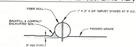
FIBER ROLL SEDIMENT BARRIER (SECTION)
