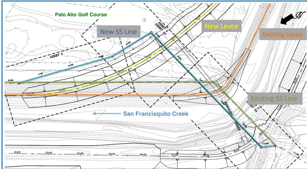
Figure 5 Planned Dewatering Areas, East Palo Alto Sanitary Sewer (SS) Siphon Relocation Project, San Francisquito Creek Flood Control, Ecosystem Enhancement and Recreation Project
