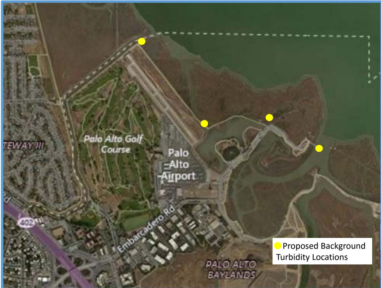
Figure 7. Location of Proposed Background Locations for Turbidity Measurements, San Francisquito Creek Flood Reduction, Ecosystem Restoration and Recreation Project, Bay to 101
