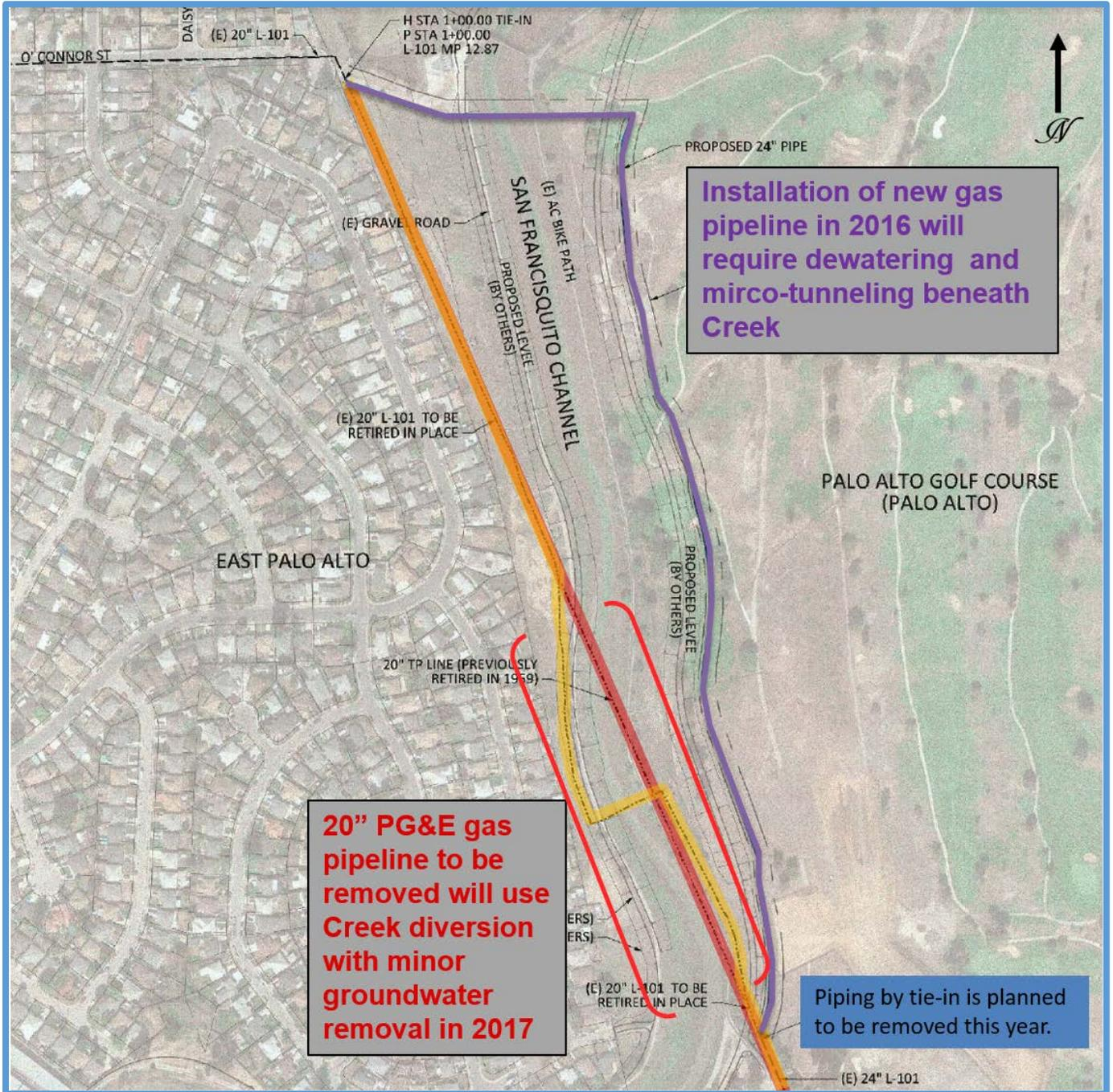
Figure 4. Planned Dewatering Areas for Gas Pipeline Relocation and Removal, San Francisquito Creek Flood Reduction, Ecosystem Restoration and Recreation Project
