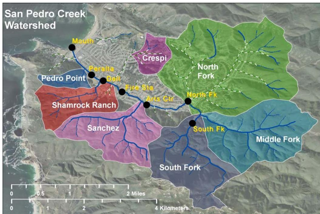
Dashed lines indicate sections of San Pedro Creek that are culverted and solid blue lines show the sections that are not.
