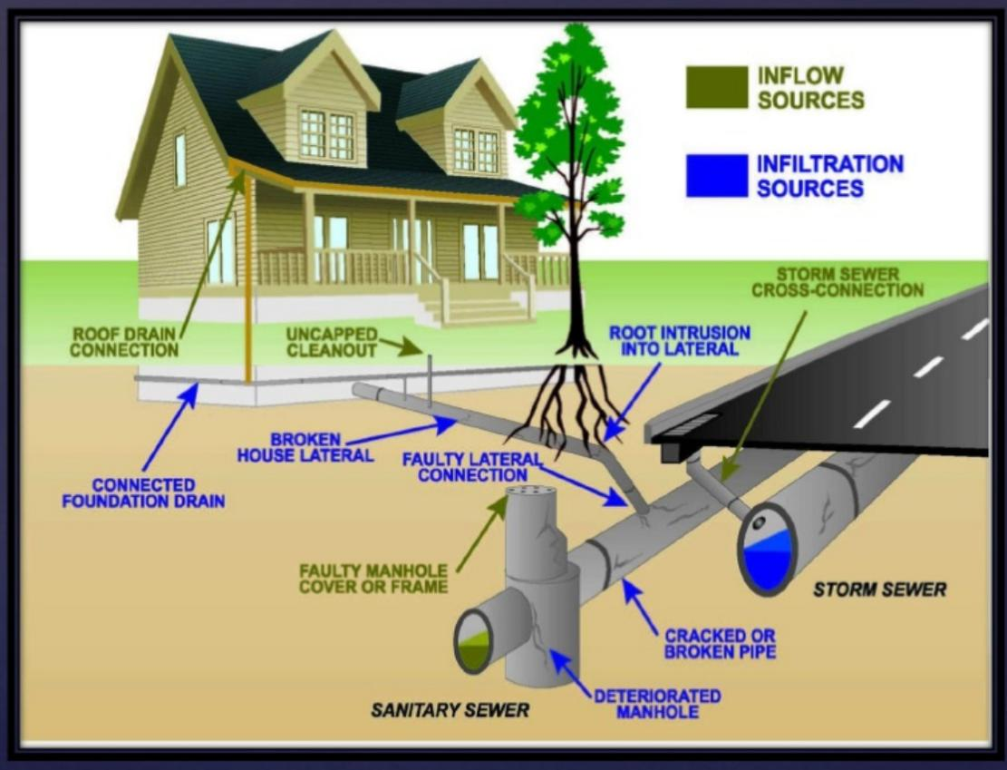
**Figure 7.7.** Example causes of inflow and infiltration
