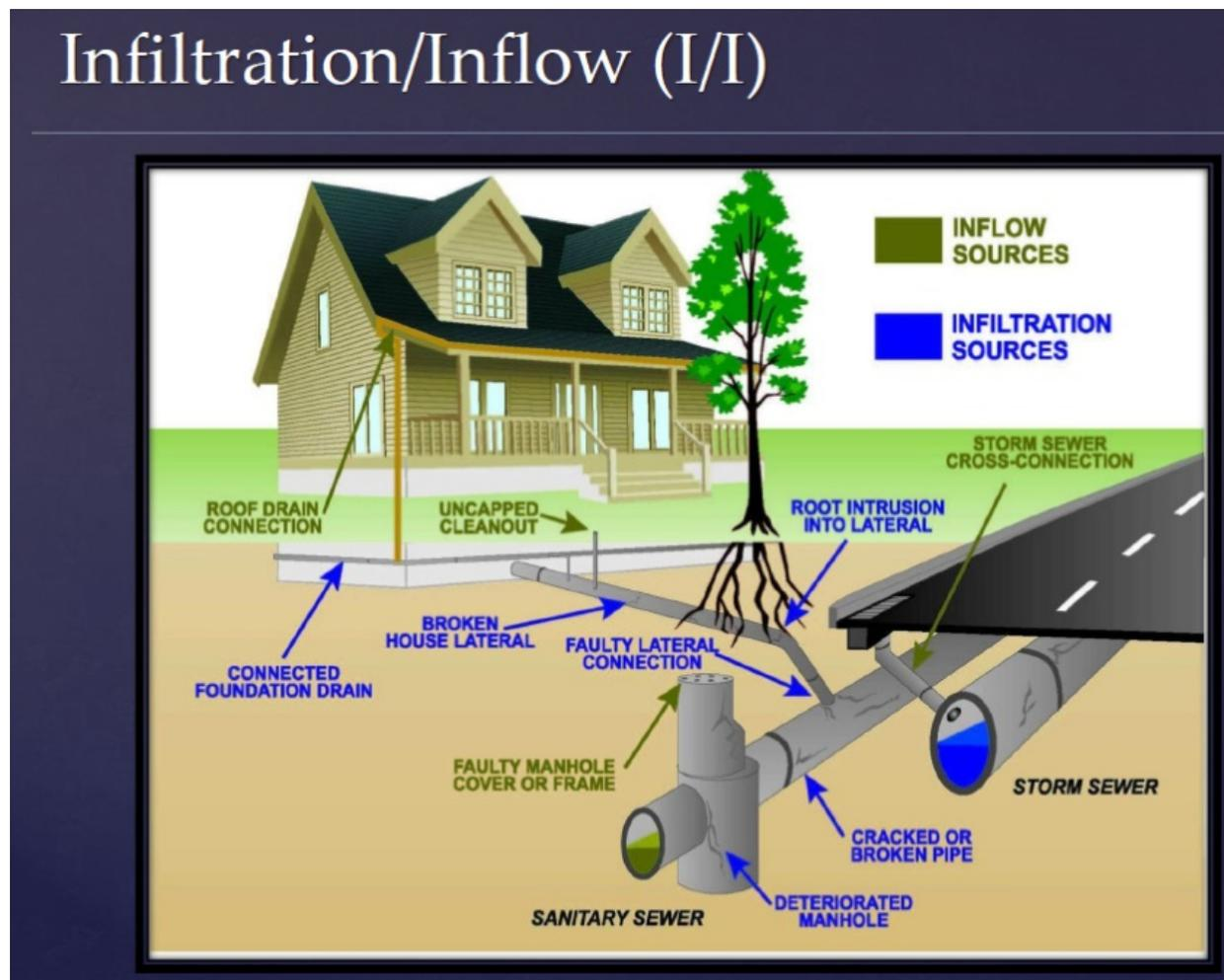
**Figure 7.7.** Example causes of inflow and infiltration.
