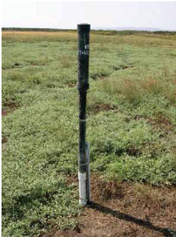
Figure 4a. Marsh Plain Installation Stilling Well (Pressure Transducer Only)
