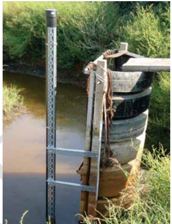
Figure 4b. Marsh Perimeter Installation Water Control Structure Stilling Well (Multi-parameter data sonde)
