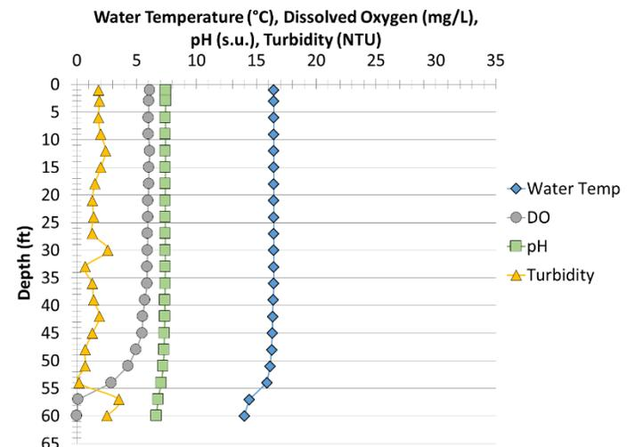
Figure 11. Dam (D-1) water temperature, dissolved oxygen (DO), pH and turbidity profiles, 2016
