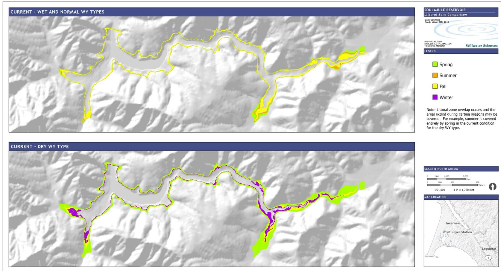
Figure 15. Spatial distribution and estimated area of the littoral zone in SoulaJule Reservoir during wet and normal water year (WY) and dry WY types under current conditions.
