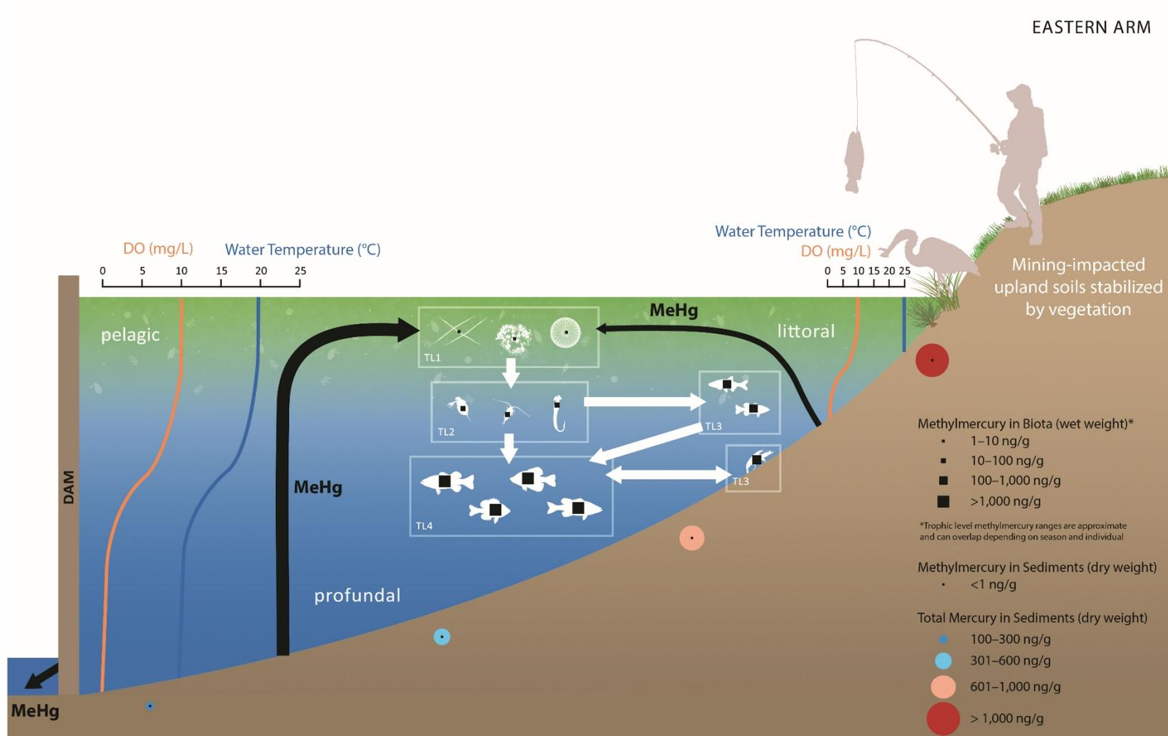
Figure 26. Existing conditions conceptual model of key factors controlling methylmercury production and bioaccumulation in SoulaJule Reservoir.
