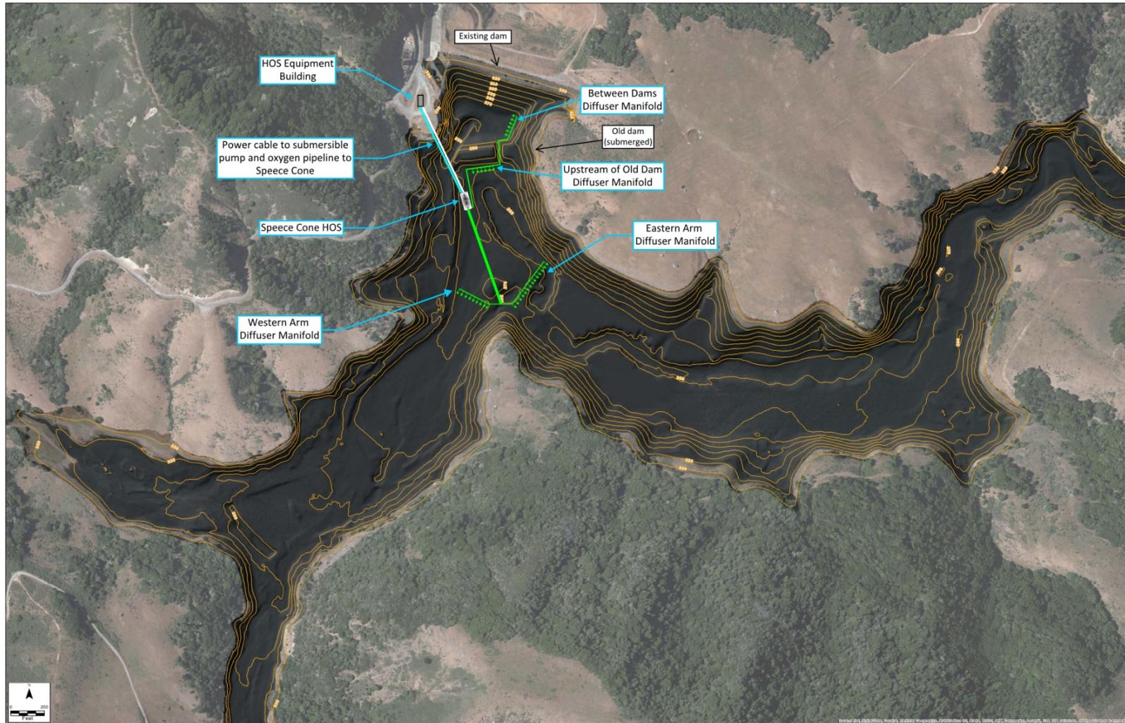
Figure 27. Preliminary in-reservoir HOS location and configuration.
