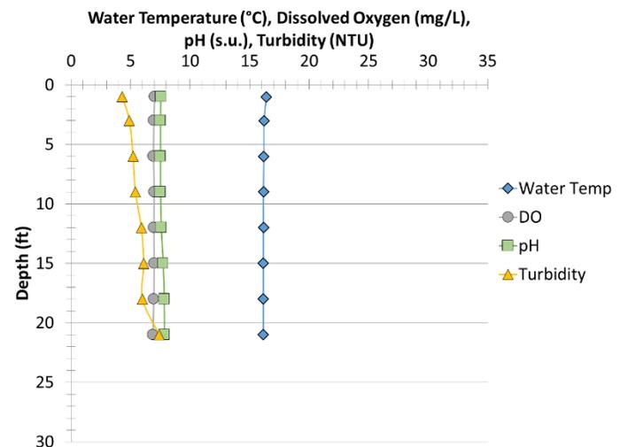
Figure 10. Eastern Arm (EA-1) water temperature, dissolved oxygen (DO), pH and turbidity profiles, 2016.
