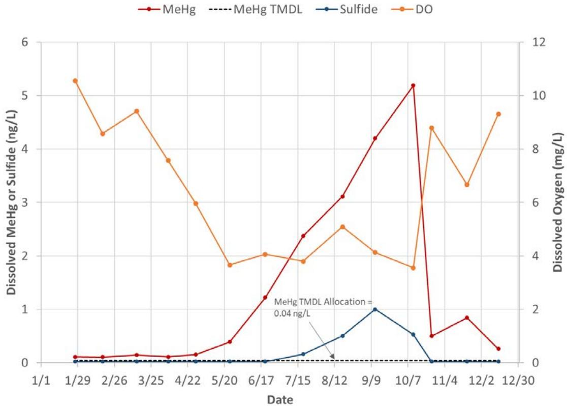
Figure 14. Monthly water concentrations of dissolved methylmercury (MeHg), dissolved sulfide, and dissolved oxygen (DO) at the dam outlet (Site AC-1).
