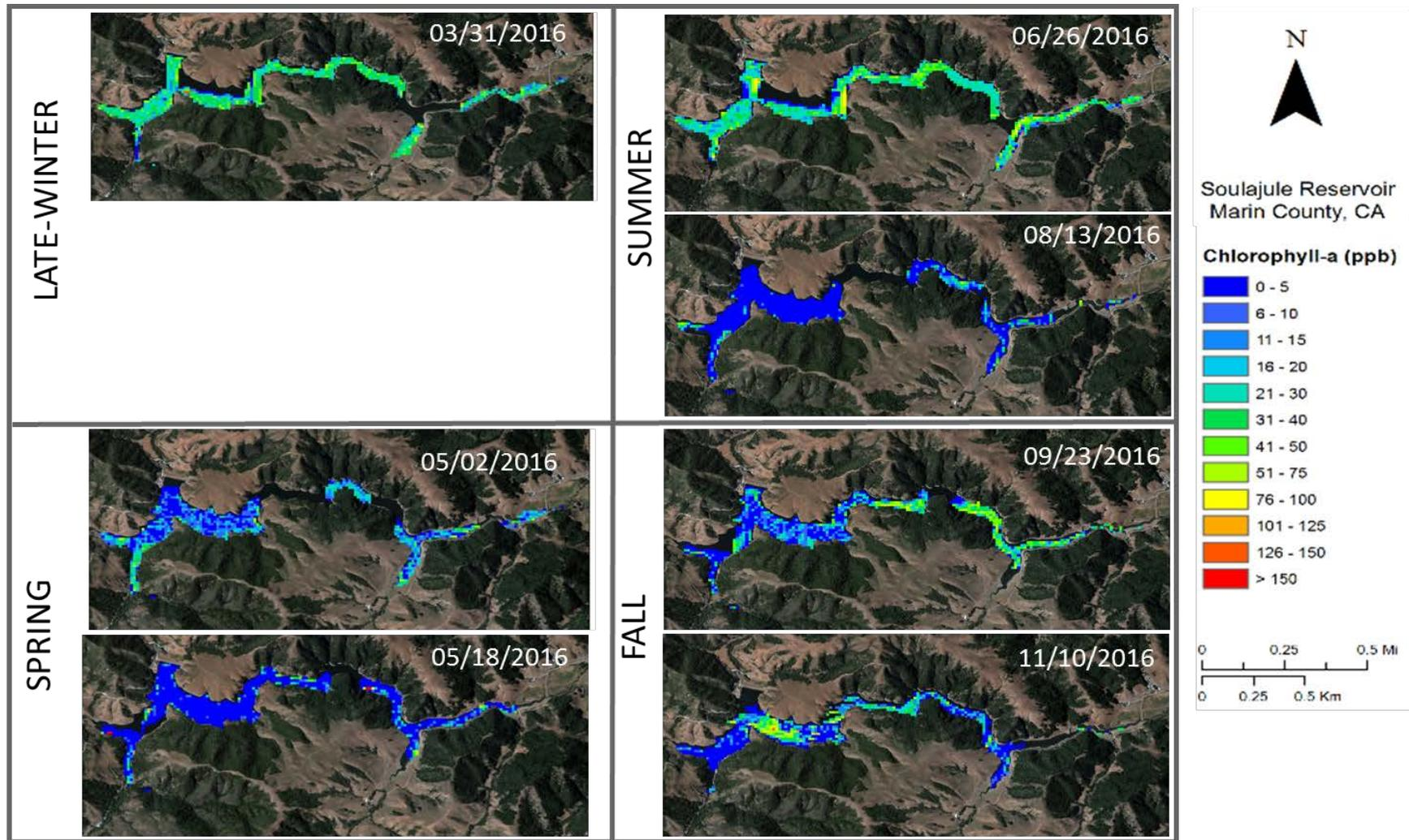
Figure 16. Chlorophyll-a concentrations on various dates in late winter, spring, summer, and fall 2016. Chlorophyll-a was measured using raw data collected by satellite (Landsat 7 and Landsat 8) imagery and processed by Satelytics (Toledo, OH).
