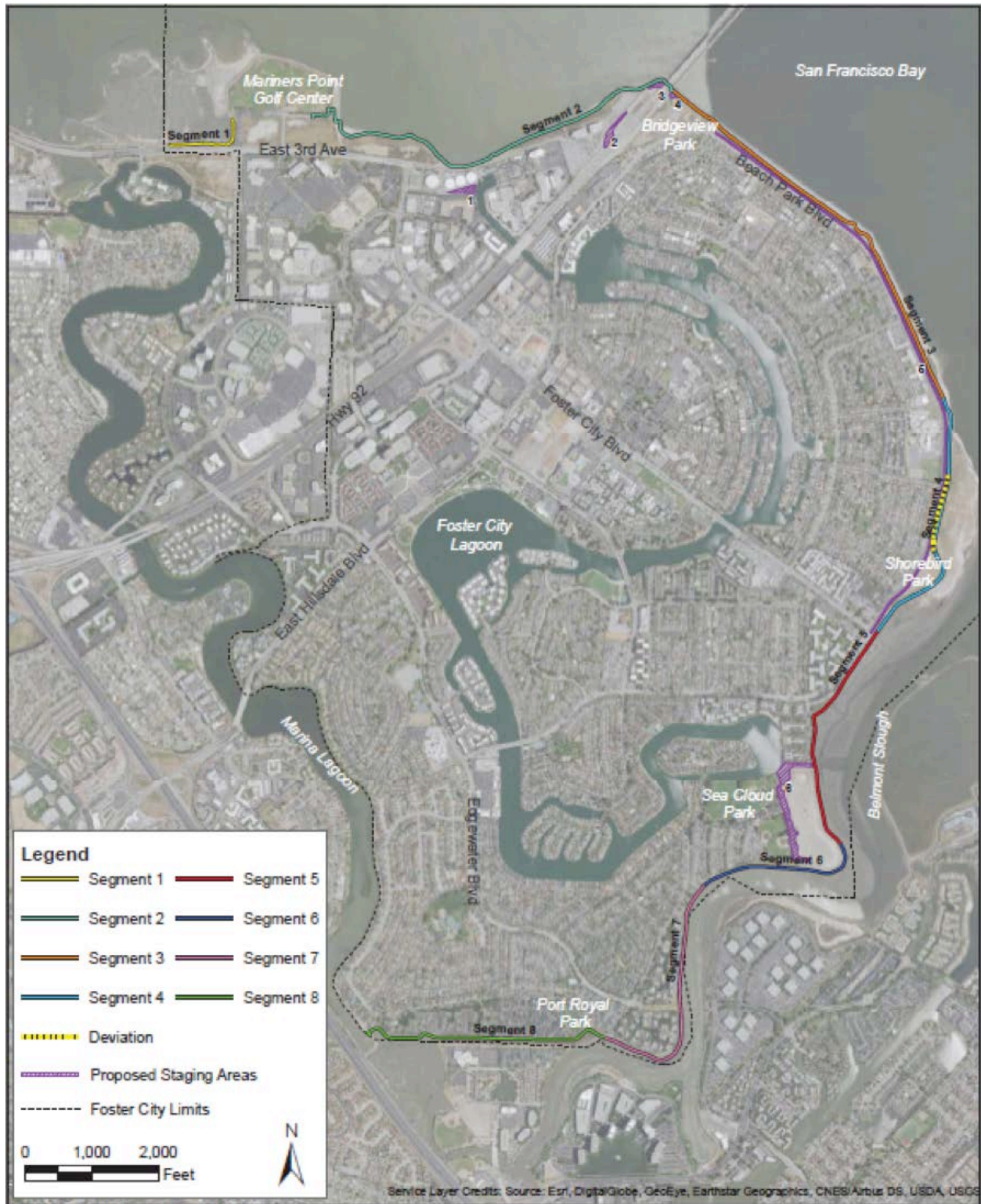
Figure 19. The levee system surrounding Foster City. Note the extensive shell hash beach outboard of the levees in Segments 3 and 4, and the tidal mudflats & wetlands outboard of the levees in Segments 1, 5, 6, and 7. (Image: Foster City)
