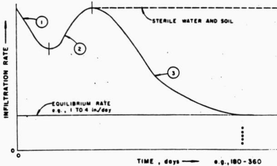
FIGURE I-3 TYPICAL TIME-RATE INFILTRATION CURVE FOR WATER (3)
