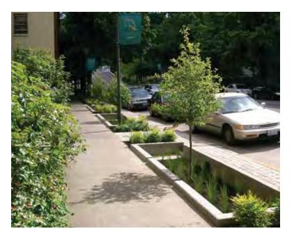
Street planters in Portland, OR, are used in highly developed urban areas to introduce green space and manage stormwater runoff. PHOTO COURTESY OF THE PORTLAND BUREAU OF ENVIRONMENTAL SERVICES
