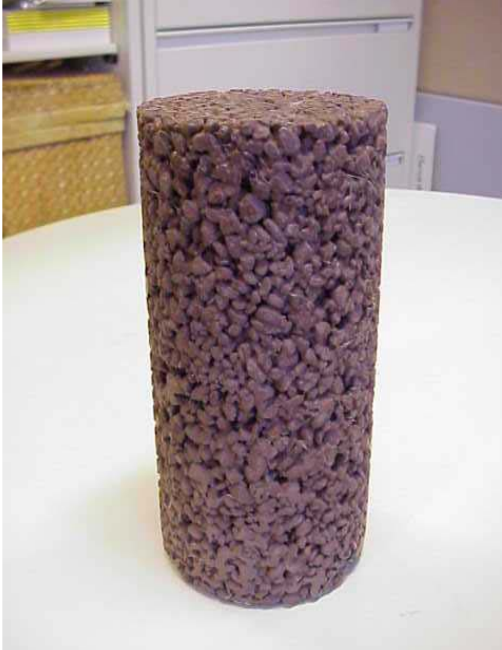
Core-Sample of Pervious Concrete, Dyed Brown
