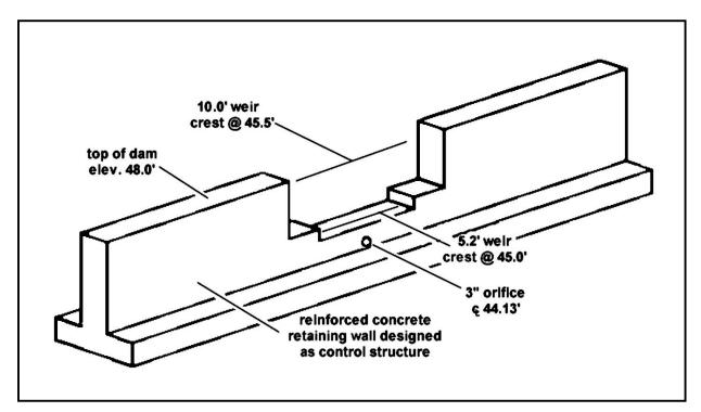
Figure C.1.5 Schematic of Control Structure
