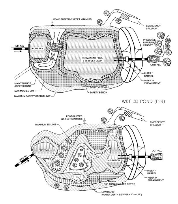
Figure A.2 Hydrologic Zones Around Stormwater Facilities
