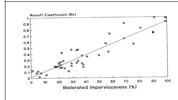
The runoff coefficient  $(R_v)$  expresses the fraction of rainfall that is converted into runoff. The data points reflect over 35 monitoring stations in the U.S.
