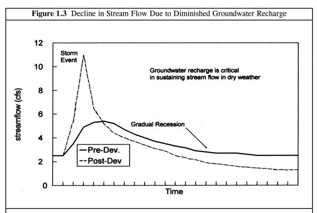
After development, stream flow declines during extended periods of dry weather because of the diminished recharge of groundwater.
