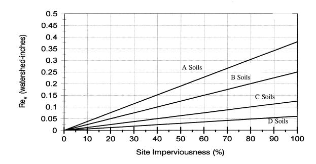
Figure 2.3 Relationship between  $Re_v$  and Site Impervious Cover
