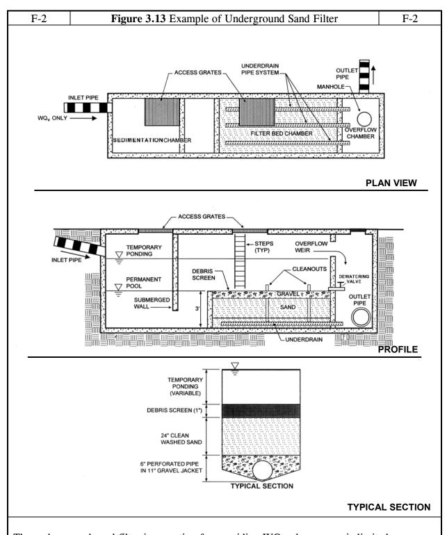
The underground sand filter is an option for providing  $WQ_{\mbox{\tiny $V$}}$  where space is limited.
