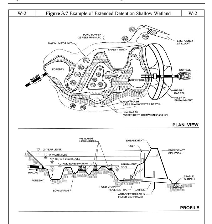
ED shallow wetlands provide water quality storage by a combination of shallow wetland pool and extended detention storage.
