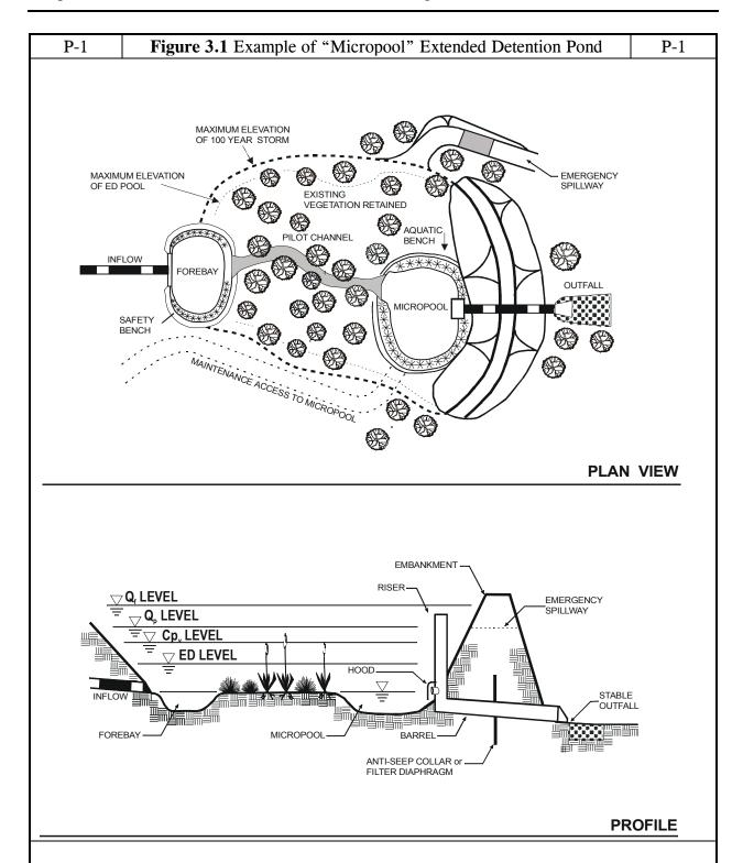
A micropool is provided in an extended detention pond to prevent resuspension of previously settled sediments and prevent clogging of the low flow orifice.
