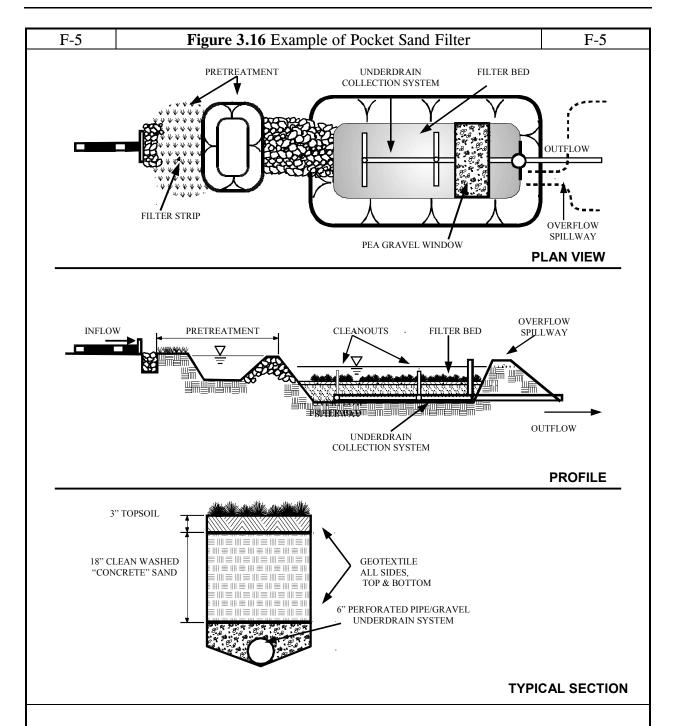
The pocket sand filter is applied to small sites where sediment loads are expected to be moderate to low. The pea gravel windows allow runoff into the filter if the surface becomes clogged.
