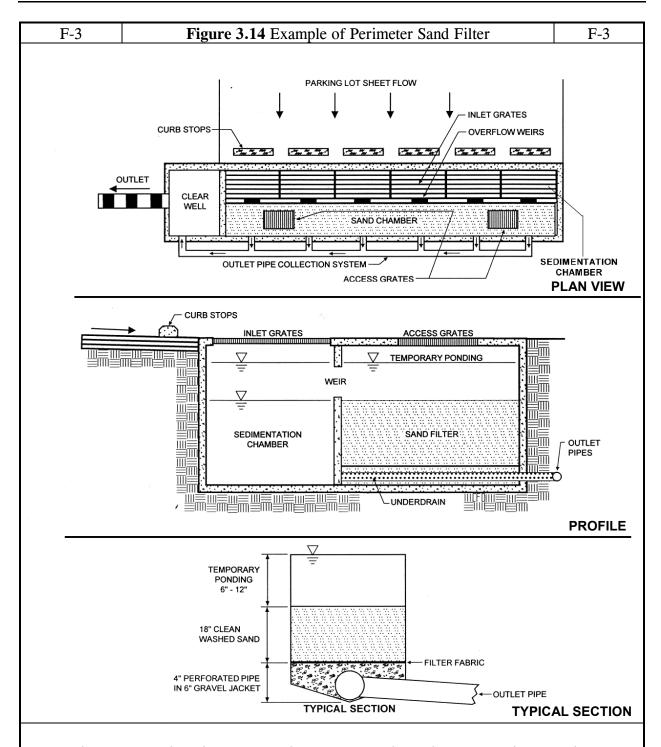
The perimeter sand filter is most practical for small sites with flat terrain or a high water table.
