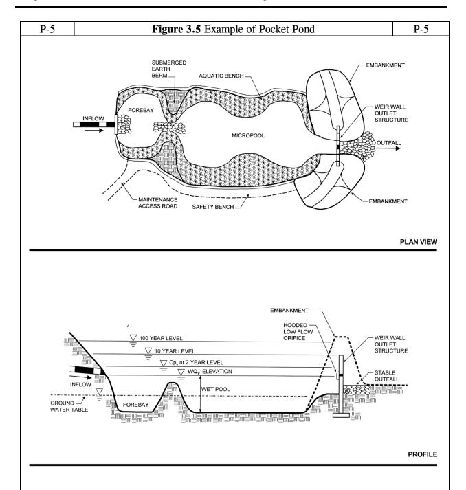
A high water table or groundwater interception maintains permanent pool level in a pocket pond. However, excavation to groundwater interception should be avoided where the land uses draining to the pond may contaminate drinking water supplies.
