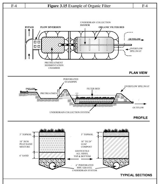
The organic filter is used when maximum nutrient or trace metal removals are desired.
