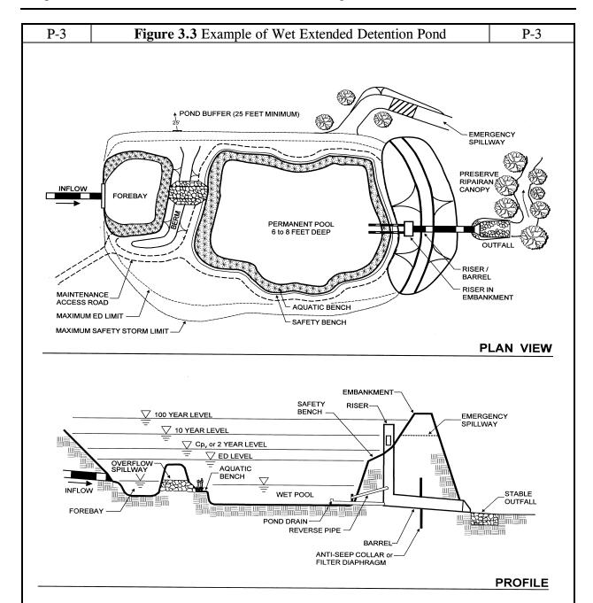
The wet ED pond provides water quality storage through a combination of permanent pool and extended detention storage.
