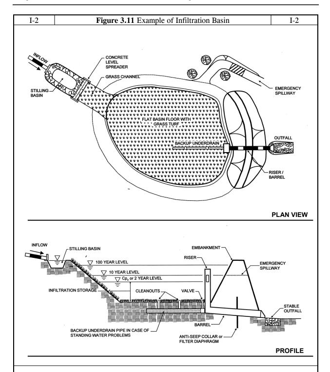
The  $WQ_{\nu}$  is retained in an infiltration basin, where it percolates through the floor of the basin in a two day period.
