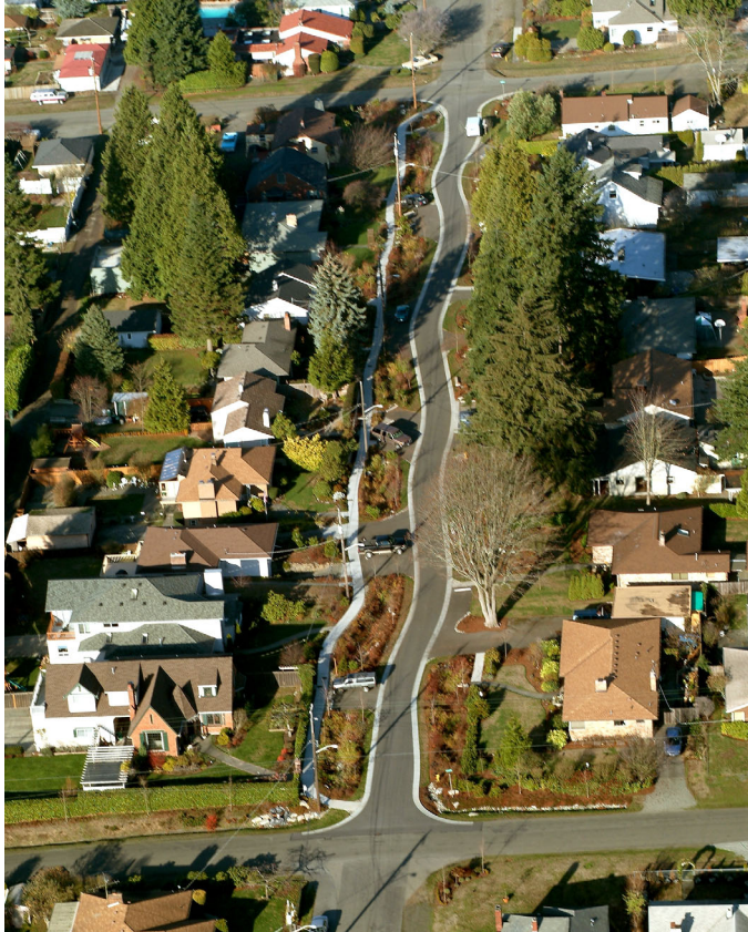
Figure 4. An aerial view of SEA street design showing narrow, curvilinear streets with sidewalks and street-edge gardens.
