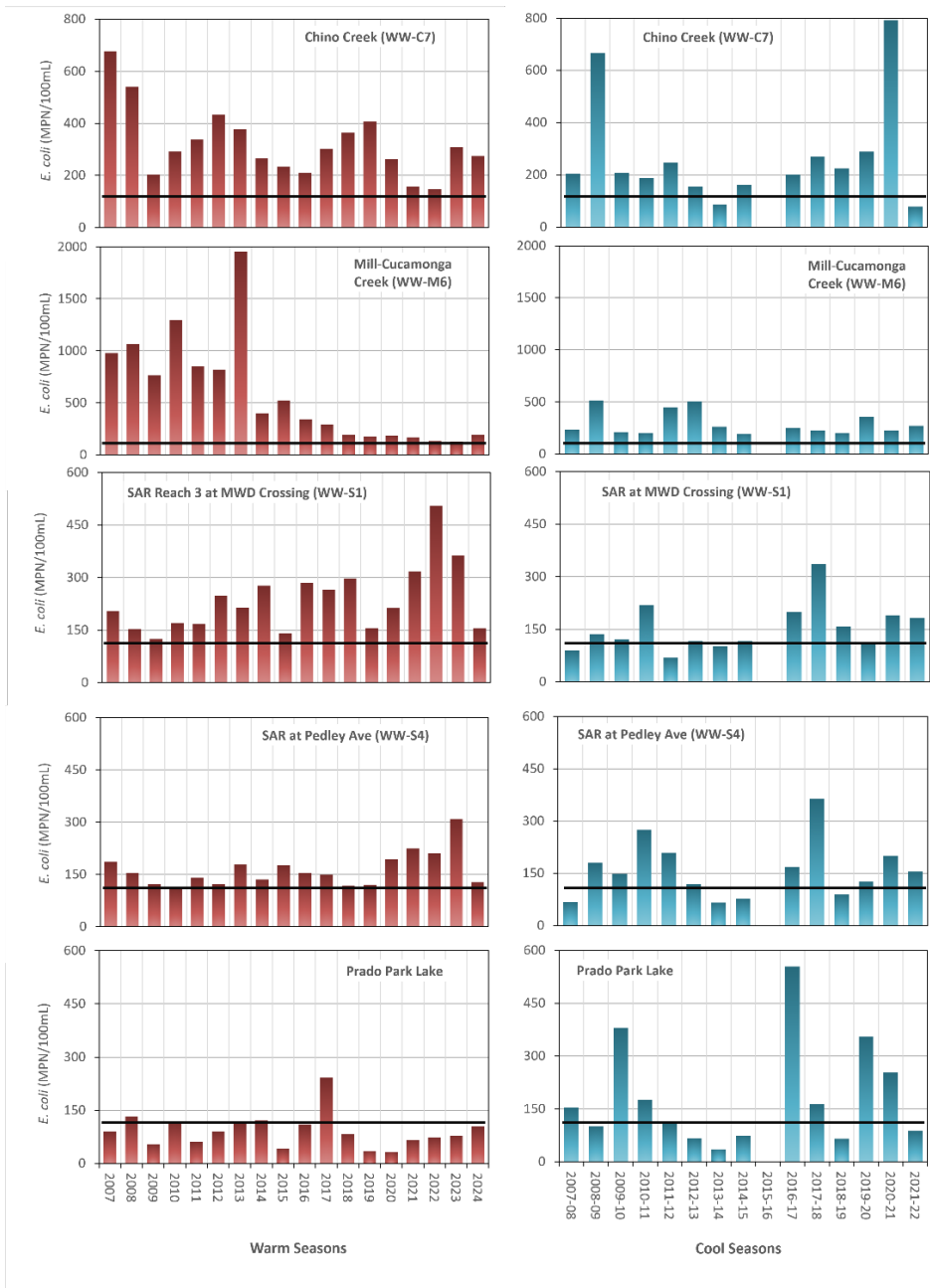
Figure 2-7. Seasonal Geomean E. coli Concentration (MPN/100 mL) for all Samples Collected at TMDL Compliance Monitoring Sites During Dry Weather in Warm (left panel in red; n = 20) and Cool Seasons (right panel in blue; n = 11 before 2016, n = 8 after 2016); the Bold Line is the Applicable WLA/LA = 113 E. coli /100 mL (SAWPA, 2023a).
