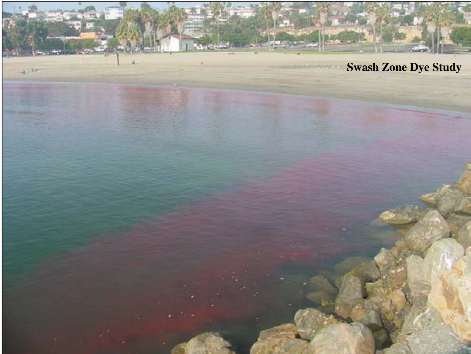
Figure 26. Dye Movement from Swash Zone in Nearshore Area Under Very Light Southwest Wind Conditions in Early Morning, 09:00 August 27, 2003, Wind 4 mph. 250-270 Degrees.
