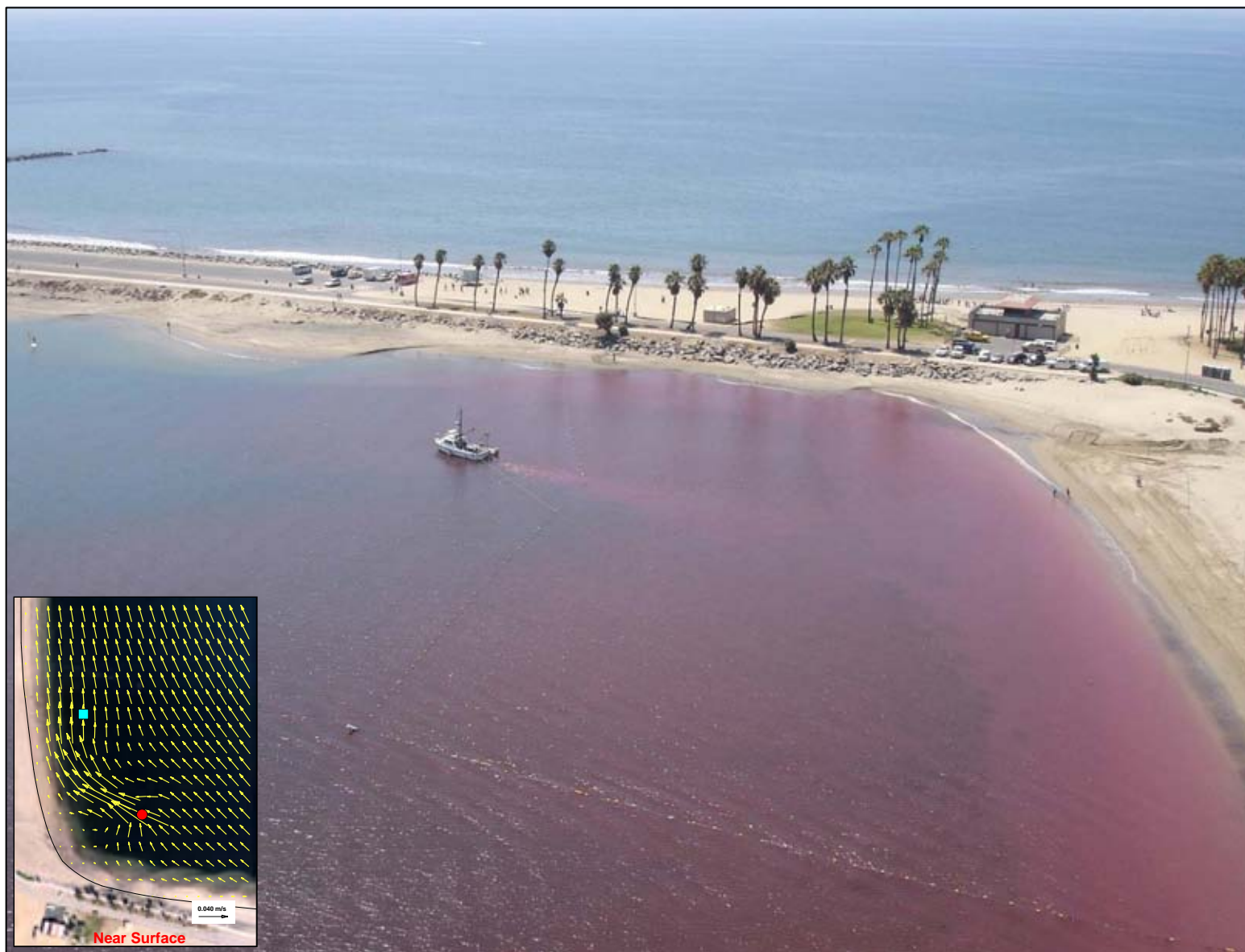
Figure 34. Aerial Photograph of Dye Distribution Southern Part of Inner Cabrillo Beach, 11:30, August 3, 2005. Insert RMA Model Predictions. (Note Pumping Started at 08:22). Red Indicates Clean Water Flushed to Beach
