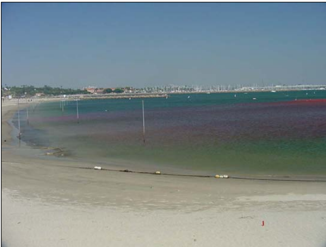
Figure 21. U.S. Corps of Engineers Dye Plume Under Predominate West Winds Inner Cabrillo Beach, 15 September 2002. Surface Layer Dye Plume Moves Offshore (top) and Transported to Beach by Bottom Countercurrent (bottom).
