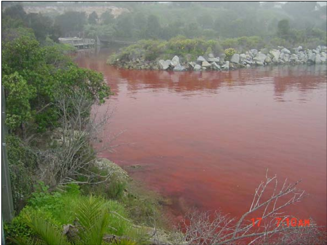
Figure 24. Rhodamine Dye in the Inner Cabrillo Beach Wetland near the Outlet at 07:30, March 17, 2004.
