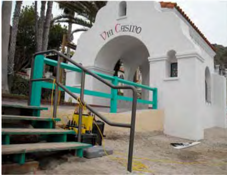
Figure 2-3. ERT set-up at Upper Step Beach, between Busy Bee Wharf and Tuna Club, at the upcoast (northwest) end of Avalon Main Beach.
