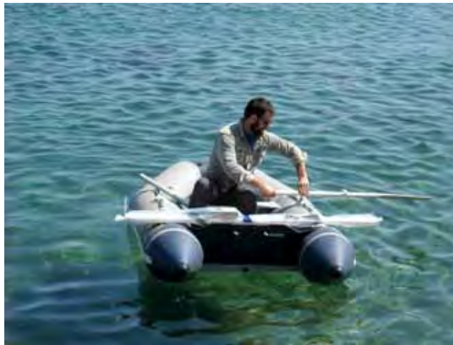
Figure 2-2. MER survey being conducted in Avalon Bay by research assistant Jordan Monroe. In this picture, the GEM-2 sensor is deployed across the back of the zodiac.
