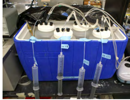
Fig. 3-1. Left: schematic of the batch experiments used to evaluate the disinfection of sewage-contaminated shallow groundwater. Right: a photograph of experimental set-up.
