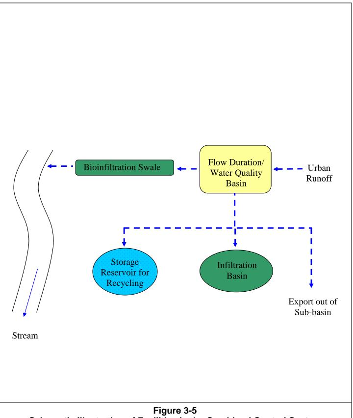
Schematic Illustration of Facilities in the Combined Control System
