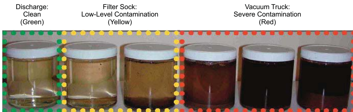
Figure 2-1: Water Contamination Grading Standard
