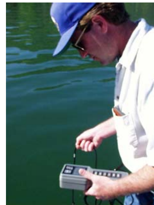
County staff collecting D.O. and Temperature readings associated with Aquatic plant management activities.
