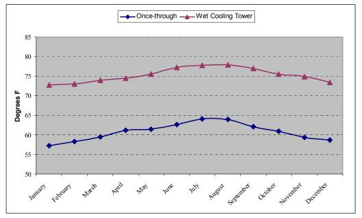
Figure K-7. Condenser Inlet Temperatures
