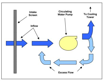
Figure K-5. Schematic of Intake Pump Configuration
