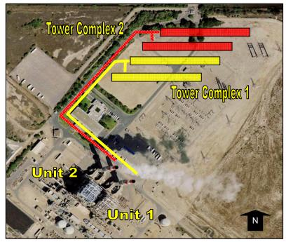
Figure K–5. Cooling Tower Locations
