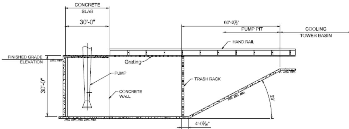
**Figure 6 – Proposed Circulating Water Pump Pit (SK-C-8)**
