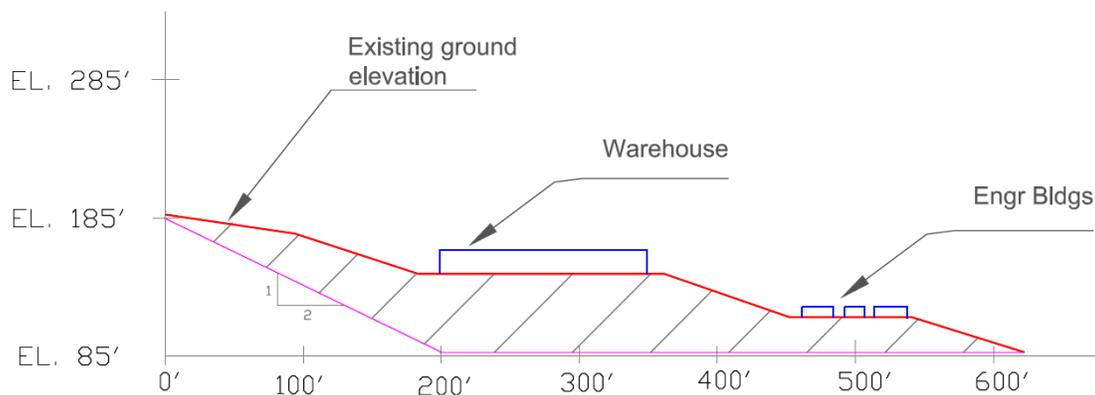
**Figure 5 – Cross Section Showing Required Excavation**
