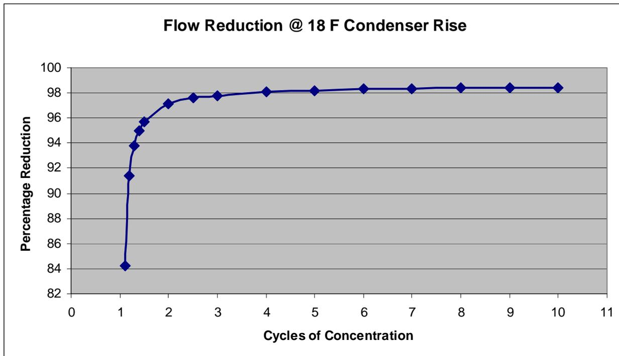
**Figure 15. Flow Reductions at Different Cycles of Concentration**
