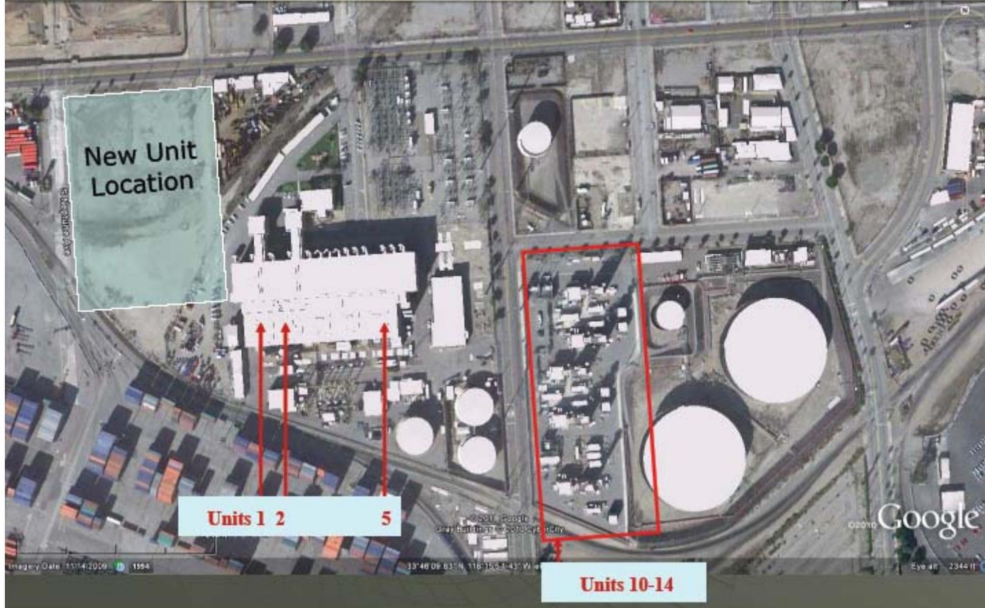
Figure HGS4 – Aerial View of Harbor Generating Station showing the Proposed Repower Layout
