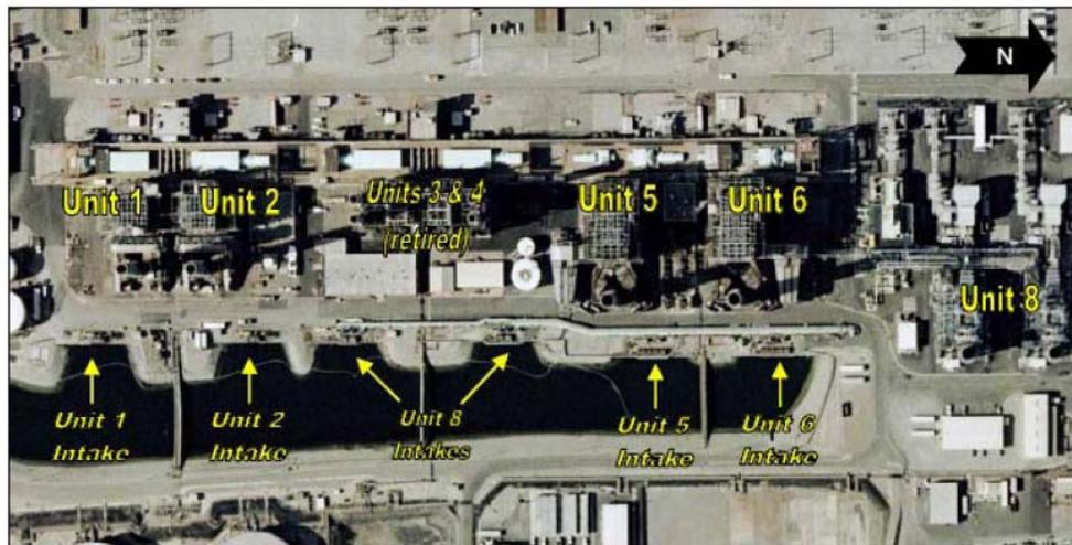
Haynes Generating Station – Generating Units and Cooling Water Intake Locations
