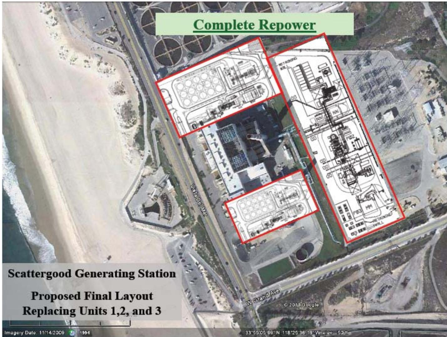
Figure SGS8 – Aerial View of Scattergood Generating Station with Final Layout Overlay
