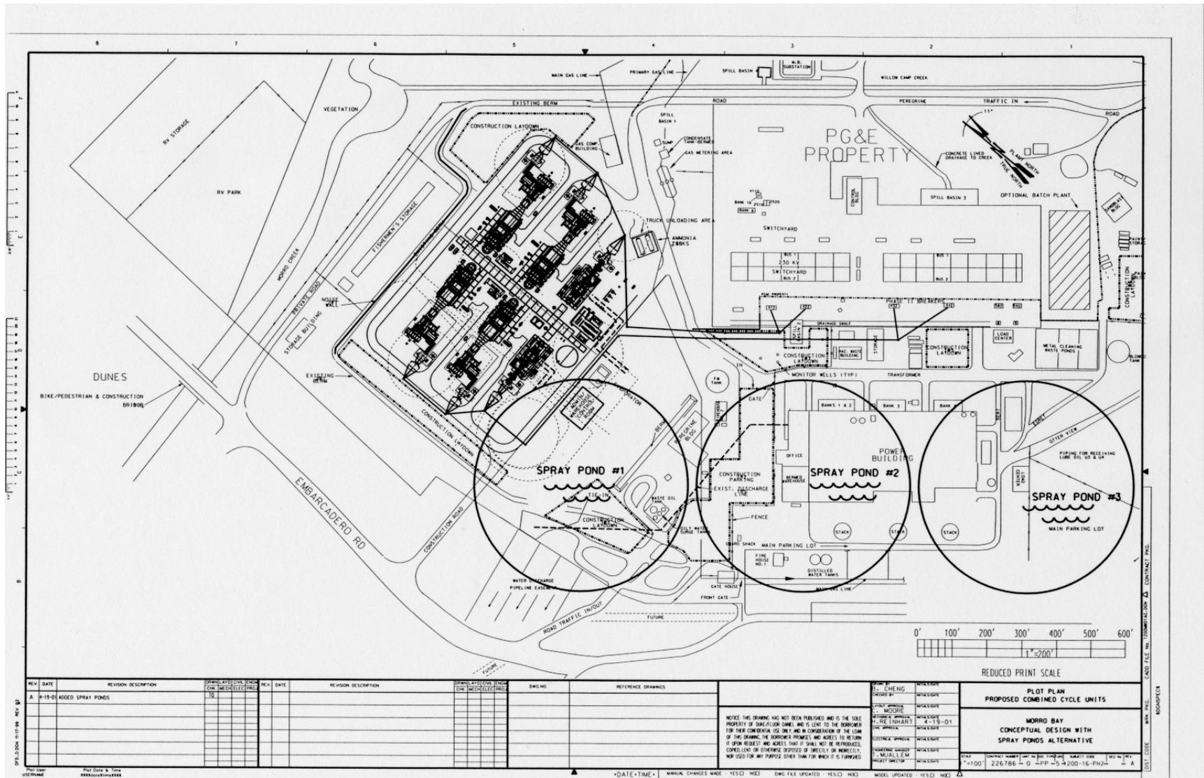
Figure 6-27. Morro Bay Power Plant alternative closed-cycle cooling spray ponds conceptual plot plan location.
