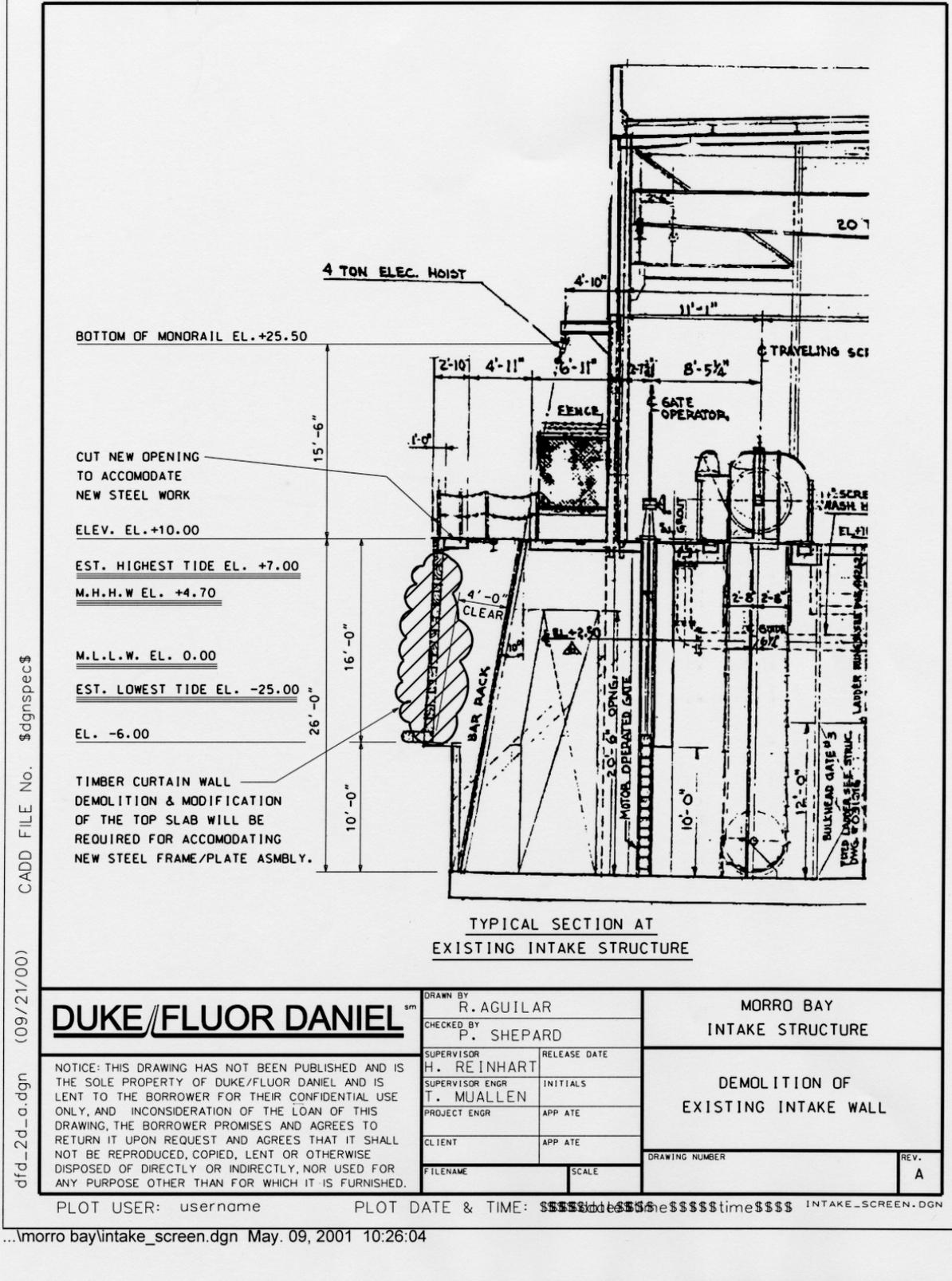
Figure 6-3. Conceptual elevation view for the vertical barrier steel assembly at the Intake structure area at MBPP.
