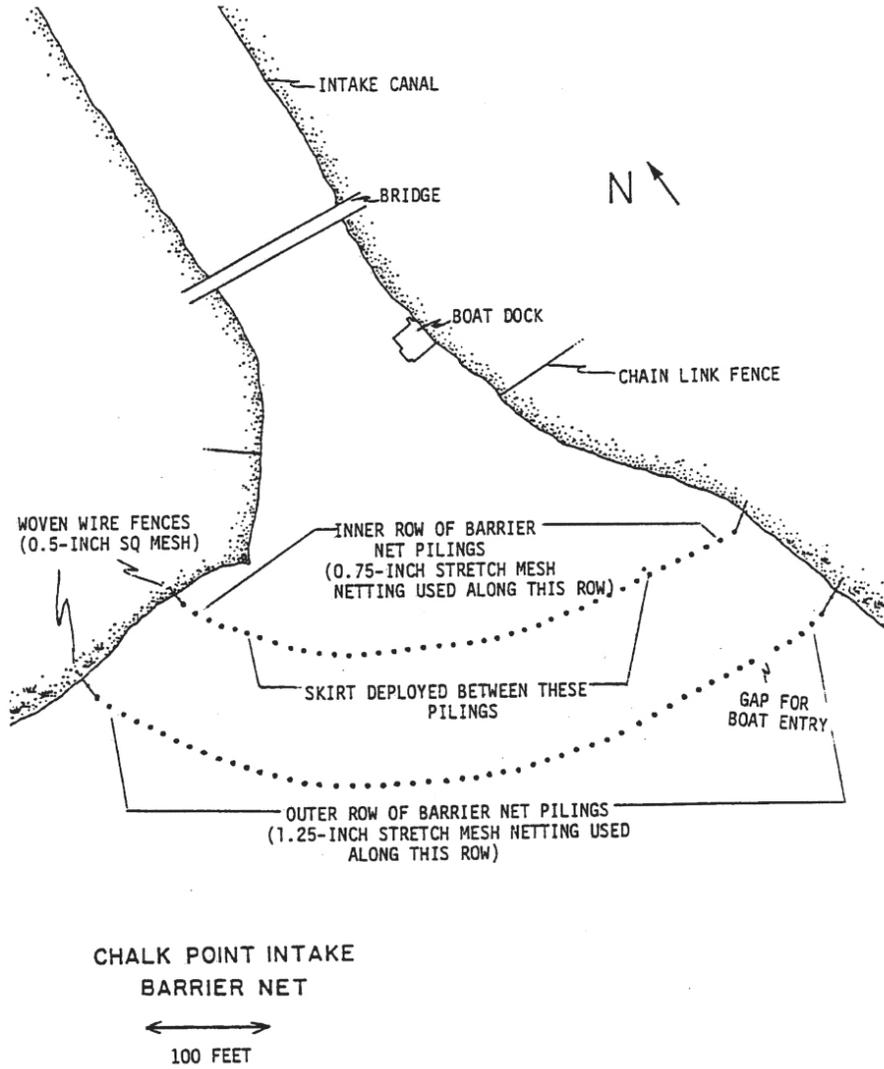
Figure 6-9. Visual example of Chalk Point Barrier Net Configuration (EPRI 1999).
