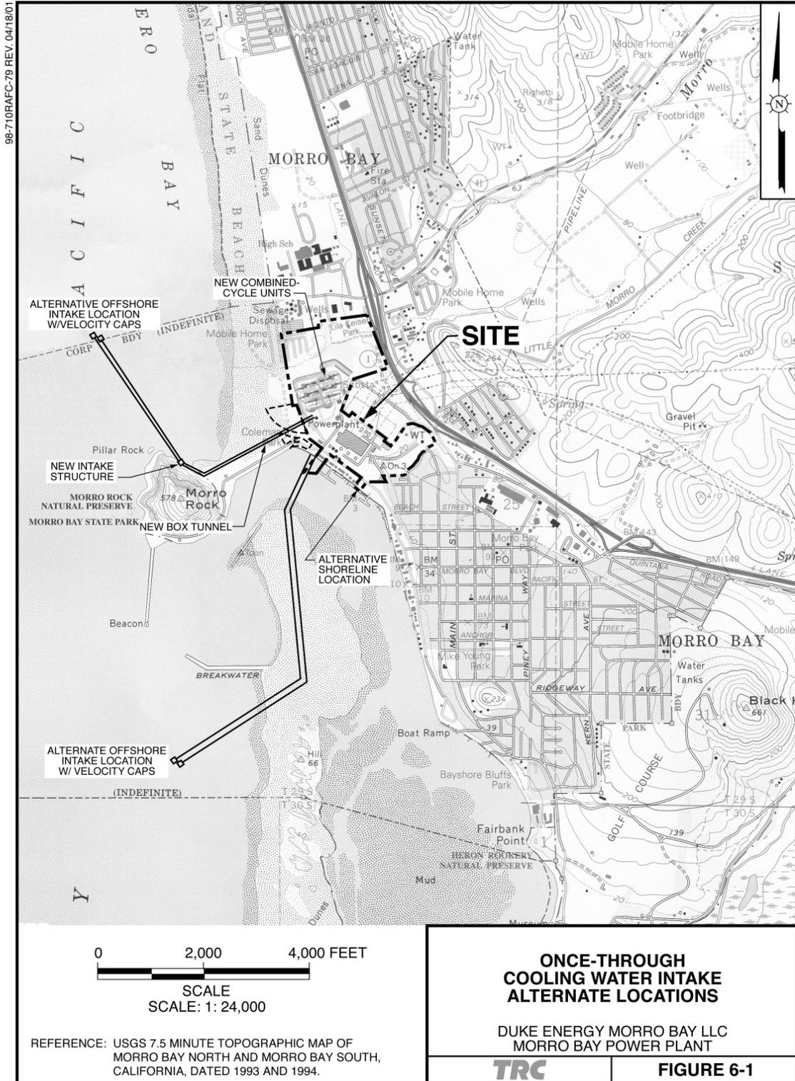
Figure 6-1. Once-through cooling water intake alternate locations.
