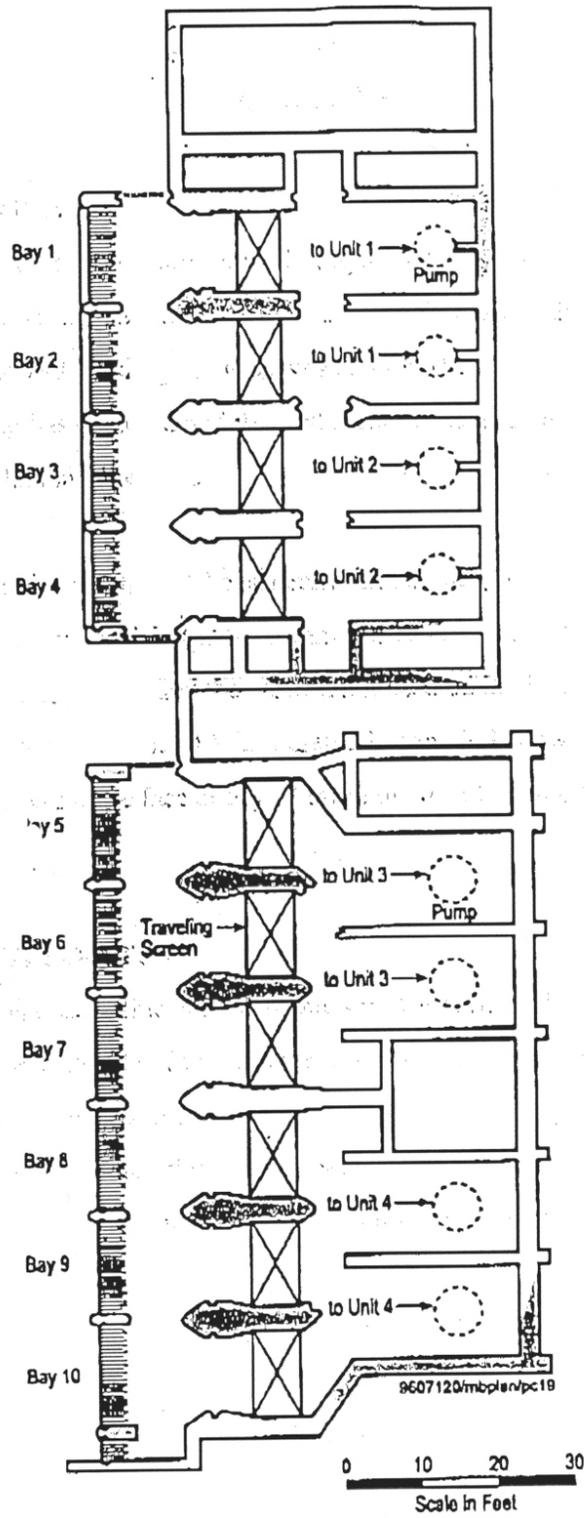
Figure 6-7. Morro Bay Units 1 through 4 intake structure, plan view.
