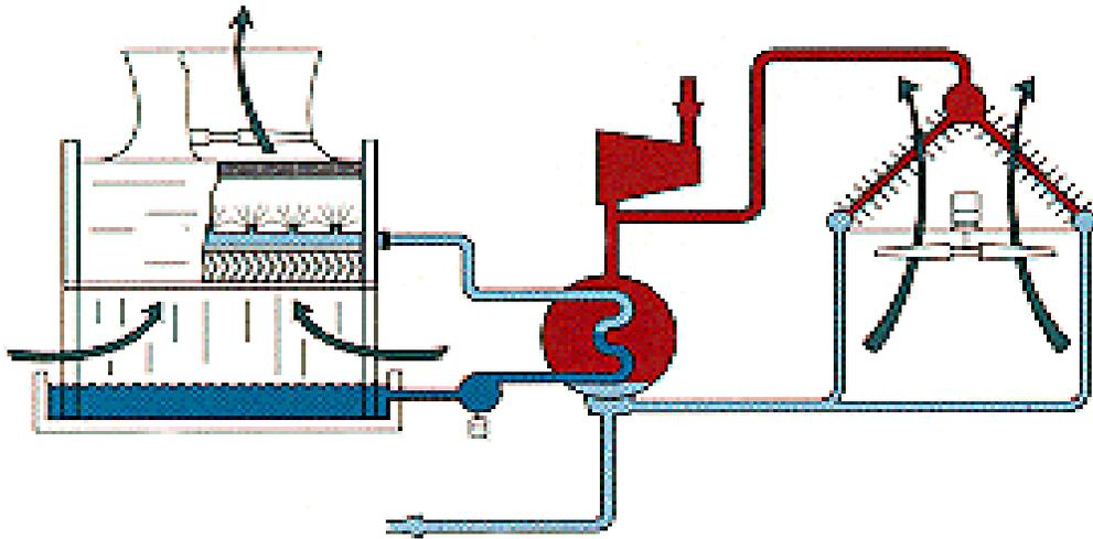
**Figure 6-25.** Schematic flow sketch of a parallel condensing system (courtesy of GEA).
