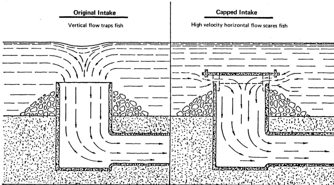
Figure 6-4. Schematic representation of an offshore structure with velocity cap (Weight 1958).
