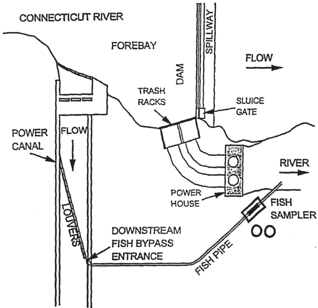
Figure 6-14. Holyoke Louver System (Stira and Robinson 1997).
