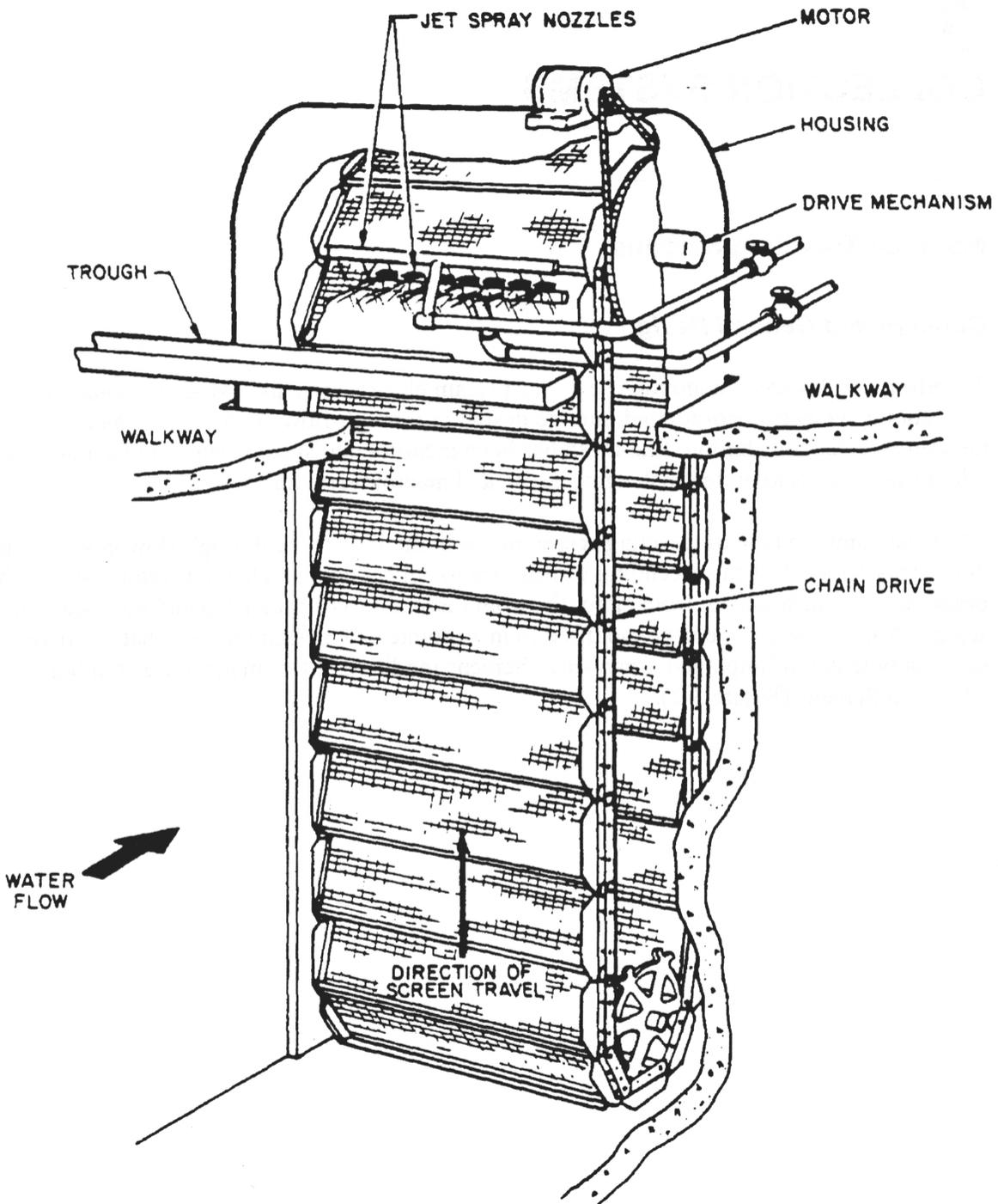
Figure 6-5. Schematic of a conventional traveling water screen (EPRI 1986).
