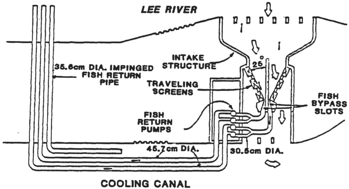
Figure 6-15. Brayton Point Station Unit 4 angled screen intake structure fish return systems (Davis et al. 1988).
