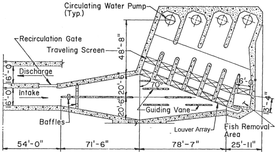
Figure 6-13. Louver System at SONGS (EPRI 1987).
