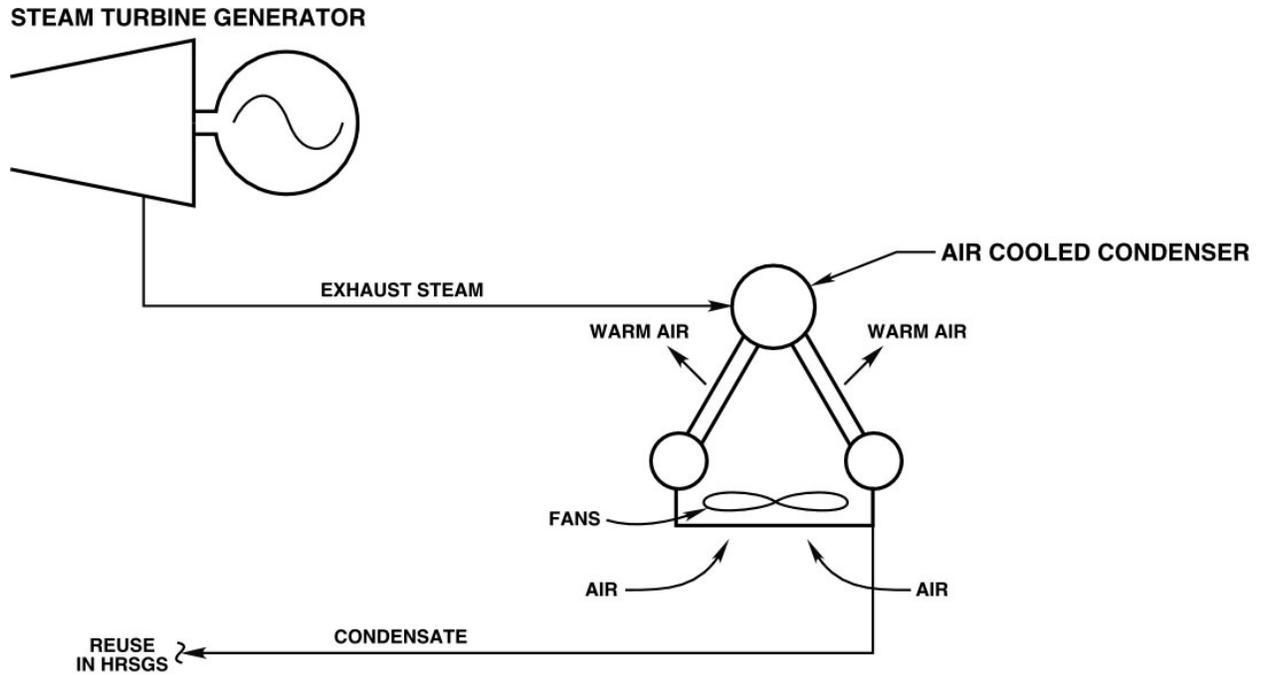
Figure 6-29. Schematic flow sketch of a direct air-cooled condenser system.
