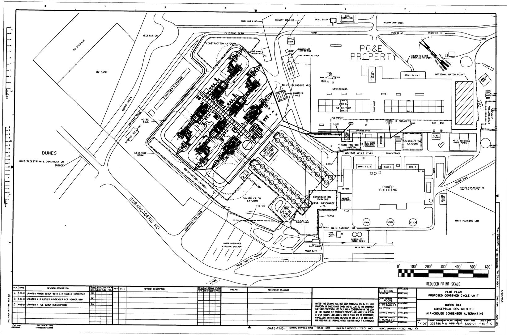
Figure 6-30. Morro Bay Power Plant alternative closed-cycle cooling air-cooled condensers conceptual plot plan location.
