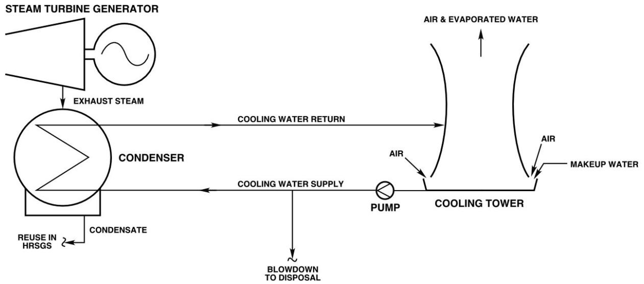
Figure 6-22. Schematic flow sketch of a natural draft cooling tower system.
