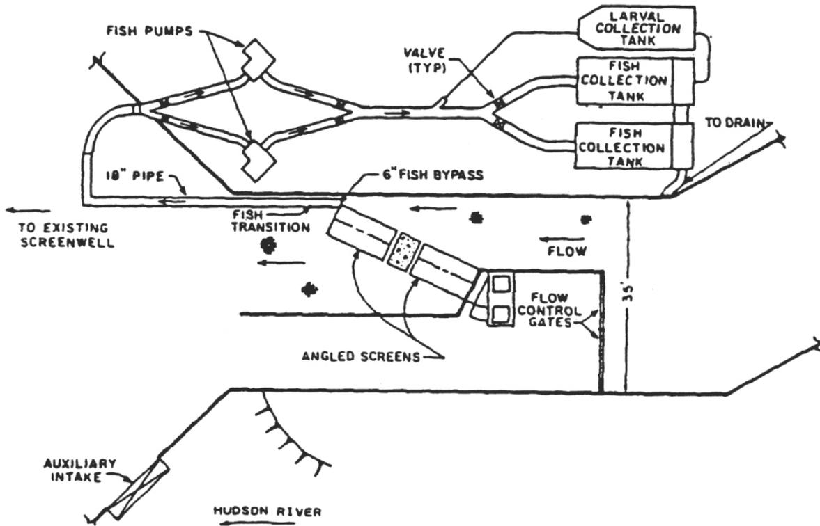
Figure 6-16. Danskammer angled screen system layout (EPRI 1999).
