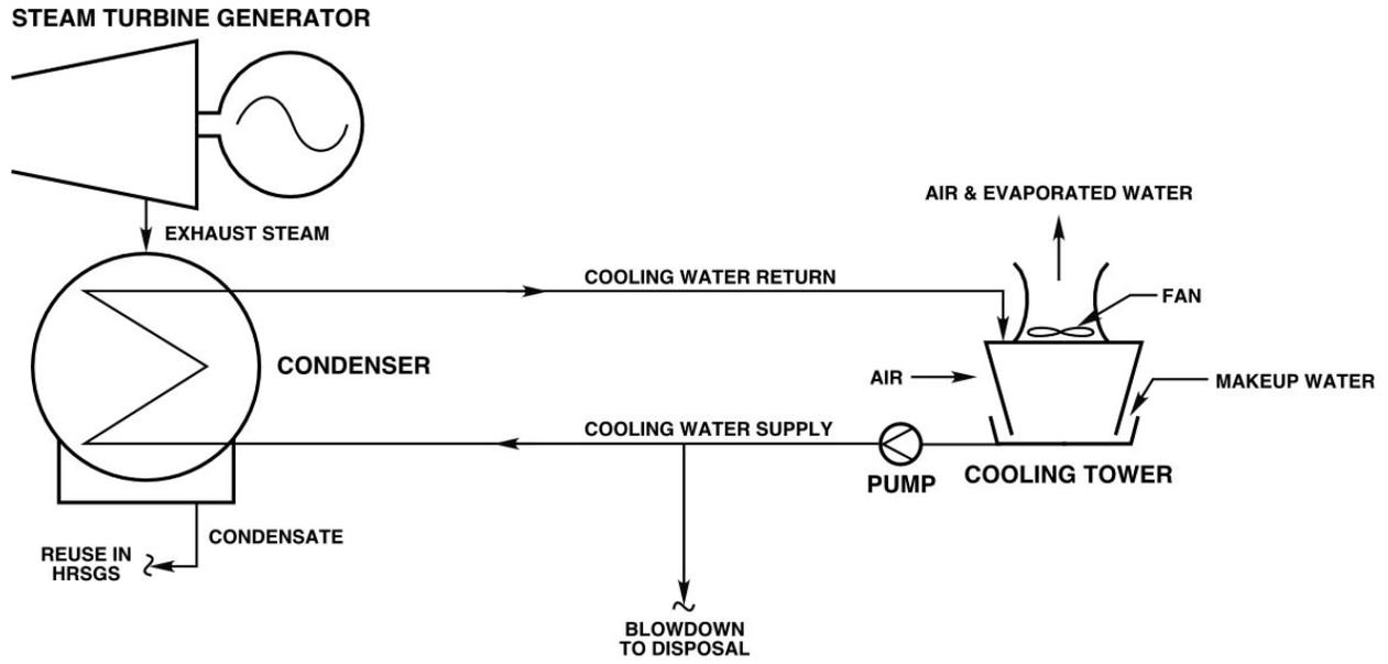
Figure 6-19. Schematic flow sketch of a mechanical draft cooling tower system.
