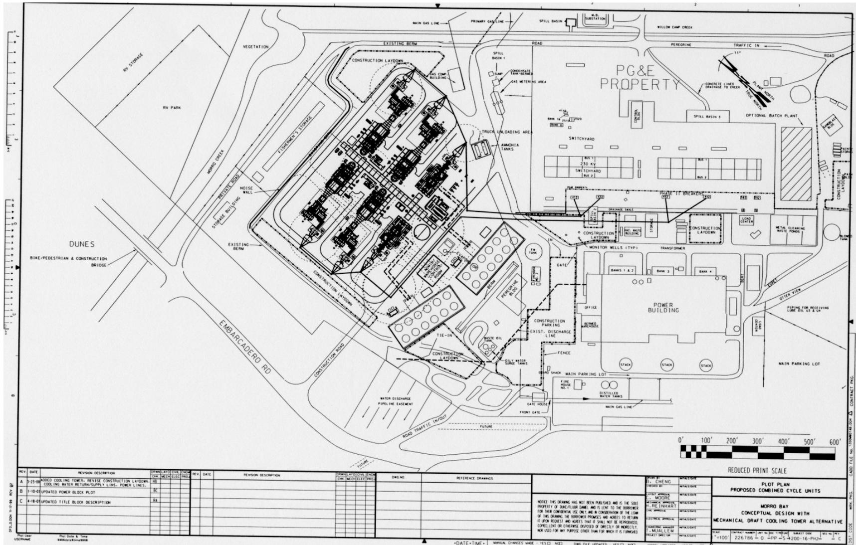
Figure 6-20. Morro Bay Power Plant alternative closed-cycle cooling mechanical draft cooling towers conceptual plot plan location.
