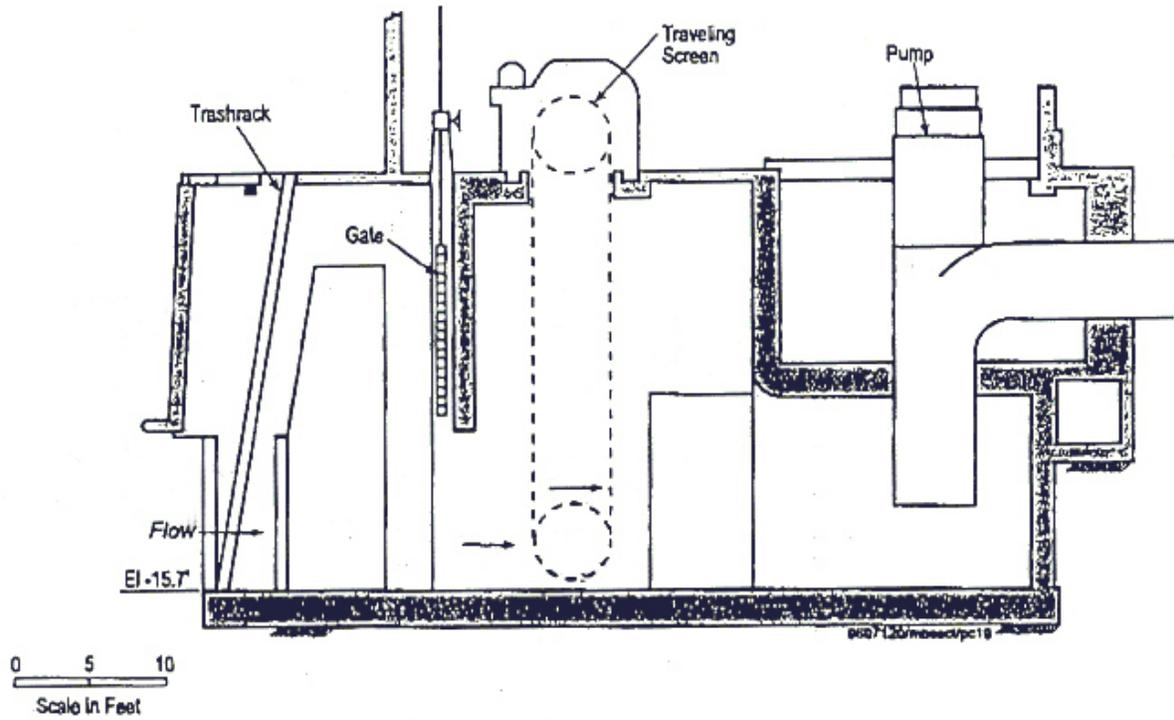
Figure 6-6. Existing Morro Bay Power Plant Units 1 and 2 intake structure, typical section.
