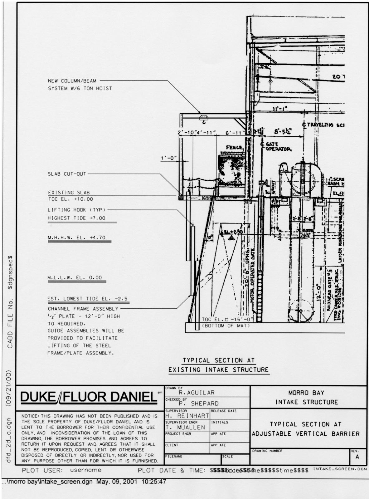
Figure 6-2. Site construction of the vertical barrier steel assembly at the Intake structure area at MBPP.
