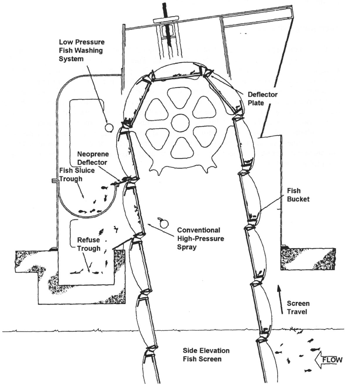
Figure 6-17. Section of a traveling water screen modified for fish protection (EPRI 1986).
