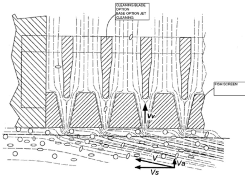
**Figure 1: AquaSweep™ and Inertial Separation**
