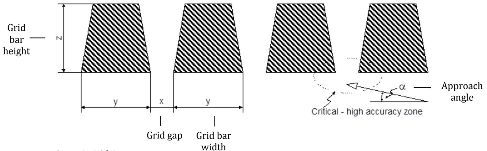
**Figure 6: Grid Geometry**
