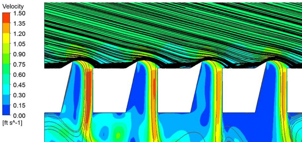
**Figure 9: Shows (100) particle tracks out of (1000) for the aquatic particle transport simulation at 4.5mm gaps with particle diameters of 1mm. No particles were pulled through the grid during the 3 second transient simulation duration.**
