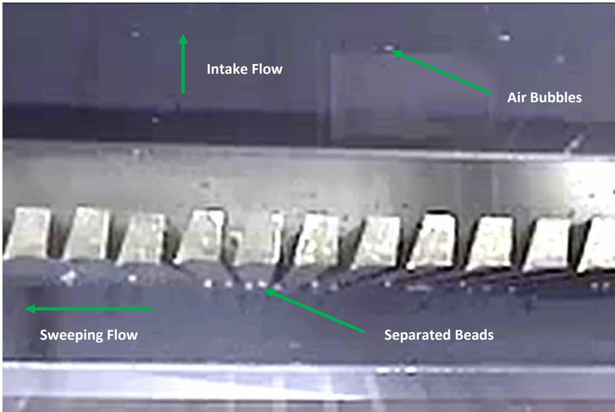
**Figure 12: 2 mm bead entrainment test**
