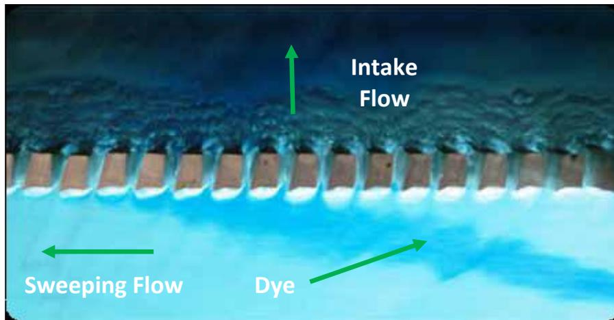
***Figure 11: Dye Test***
