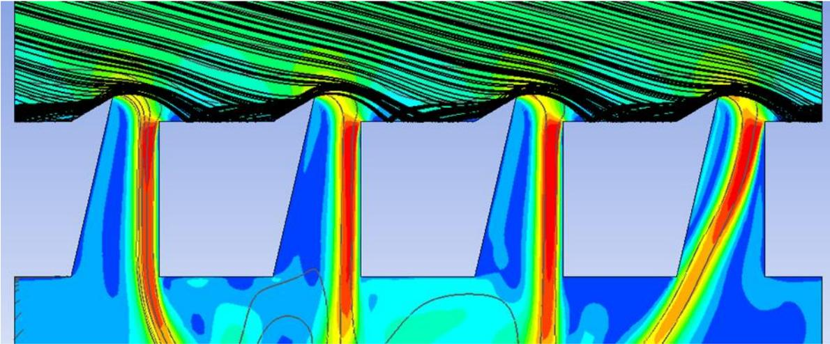
**Figure 8:** Shows (100) particle paths out of (1000) for the aquatic particle transport simulation at 3mm gaps with particle diameters at 1mm. During the transient simulation, over 3.0 seconds, the particles were shown to pass over several domains, equivalent to dozens of bar screen gaps.
