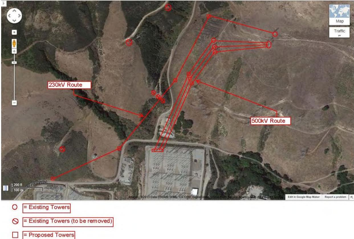
Figure 4.3-7. Existing 230 kV and 500 kV Power Line Rerouting
