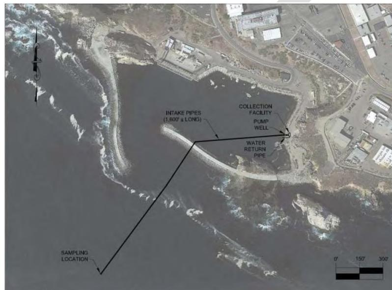
Figure A.1. Preliminary Wedge Wire Pilot Study Layout at DCPP (Reference A-1)
