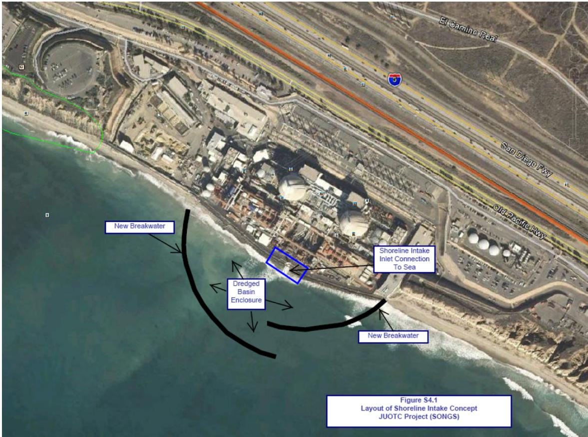
Figure IR-1. Layout of Shoreline Intake Concept
