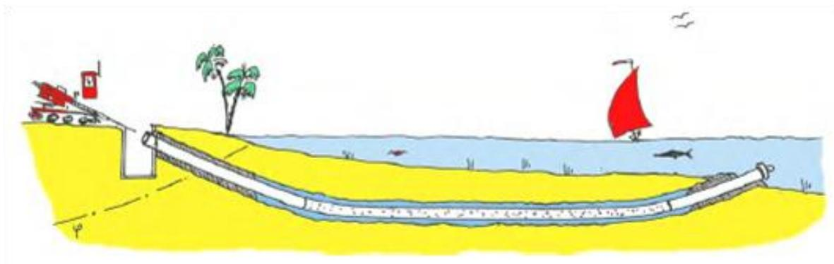
The system, called Neodren<sup>®</sup> provides extremely low turbid water as source water. Non-corrosive HDPE pipes with microporous sections (60 µm or 120 µm pores) are inserted 10 feet to 20 feet below the seafloor. The HDD laterals yield 1 to 2 MGD per lateral of source water without fish larvae, red tide algal and have no contribution or exacerbation of the seawater intruding into on the inland aquifer.
