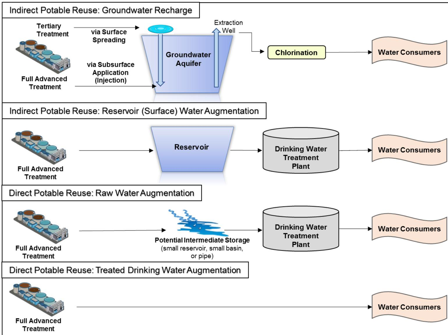
Figure 4-2 Recycled water applications for potable reuse
