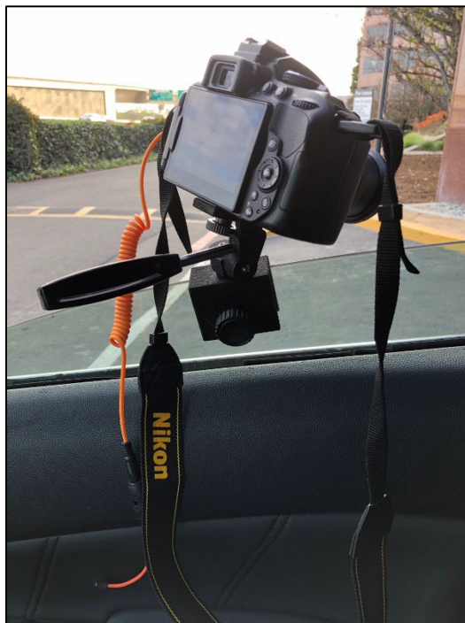
Figure 5: Proper Video Camera Window-Mount Setup
