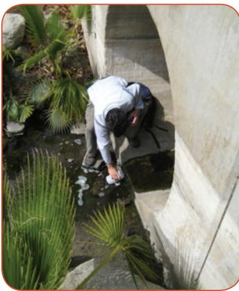
Sampling non-stormwater discharge from MS4.
