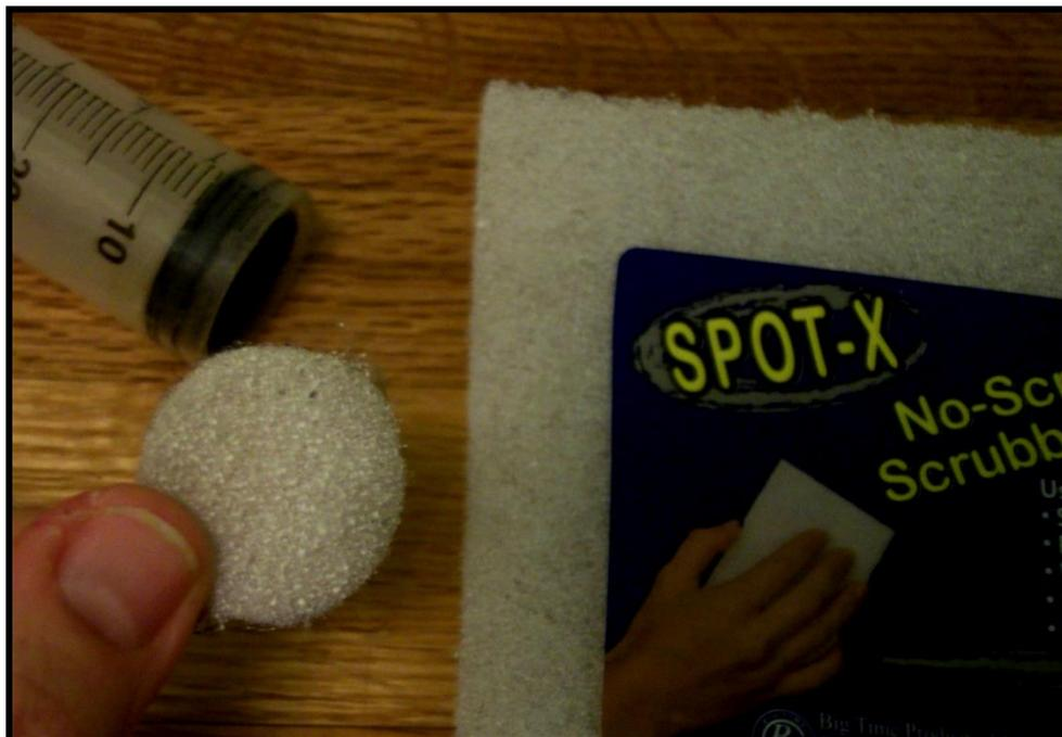
Before each sampling event, attach a fresh circular scrubbing pad to the end of the plunger. This is a head-on view of the plunger, with the scrubbing pad circle attached.
