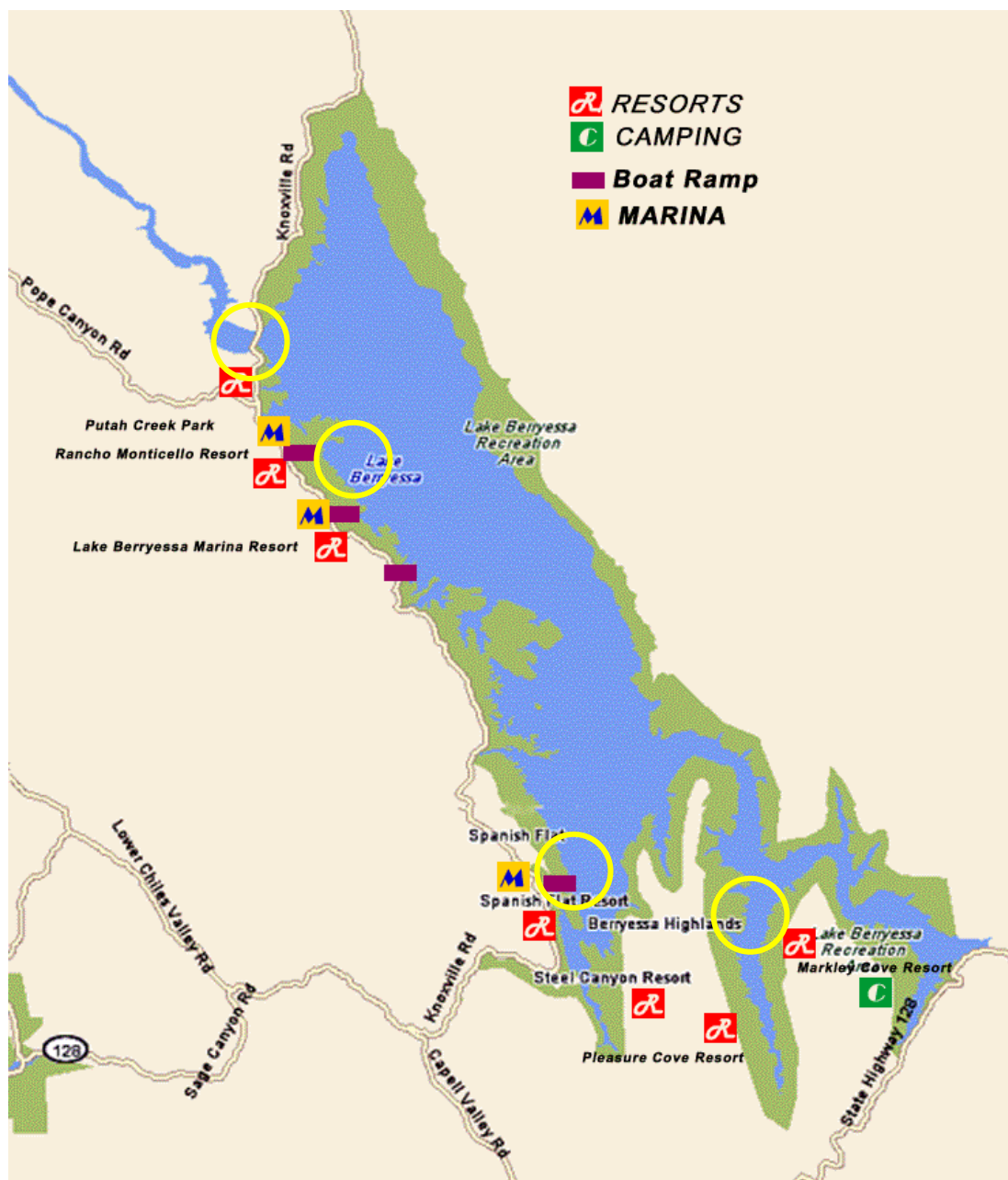
Figure 6. A representative very large lake – Lake Berryessa in Napa County. The area of the lake is 6800 ha. The width of the lake (line drawn on map) is 13 miles. Two to four sampling locations would be needed to provide an adequate sample of the lake. Diameter of circles shown is 1 mile. Locations shown are hypothetical.
