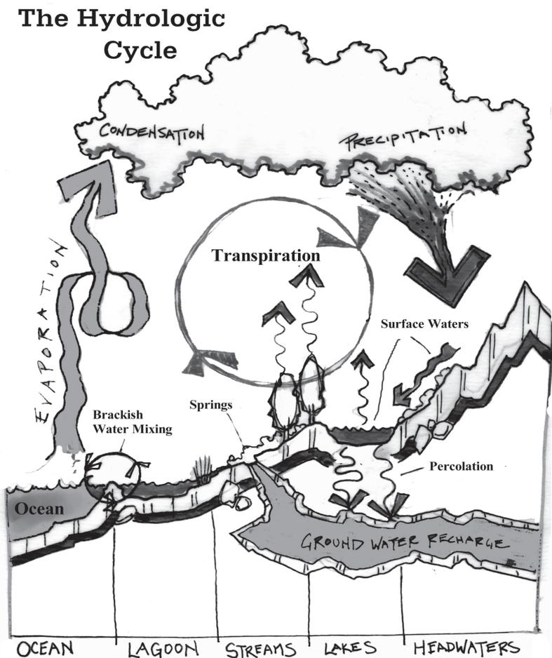
Figure 2-3: The Hydrologic Cycle
