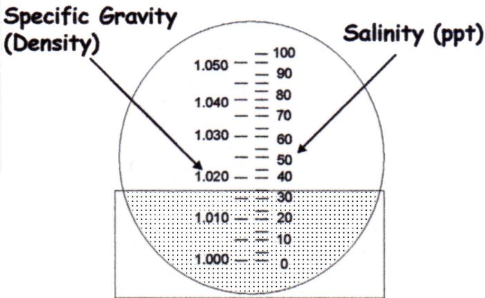
Figure 3-27: Reading the salt refractometer scale
