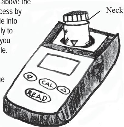
*Figure 3-3: Turbidity meter with proper alignment of indexing arrows.*
