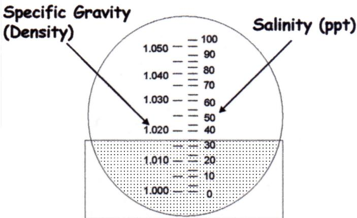
Figure 3-27: Reading the salt refractometer scale
