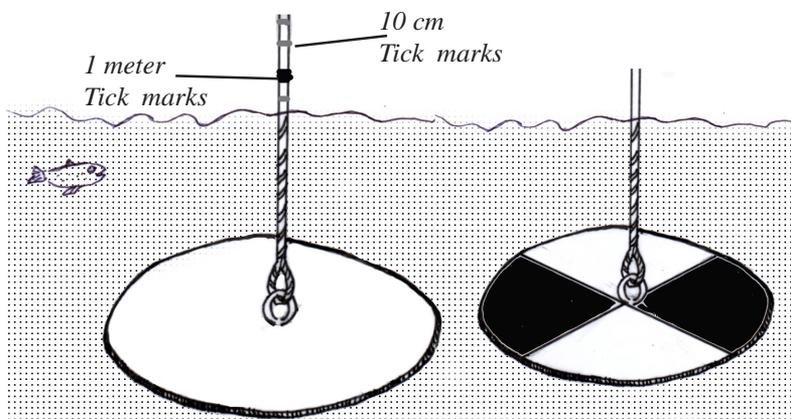
Figure 3-4: Secchi disks (White: salt water; Black and white: fresh water).
