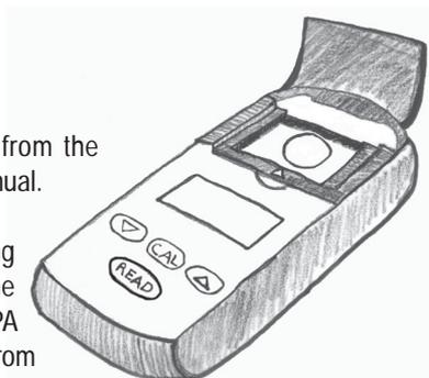
Figure 3-2: LaMotte 2020 Turbidimeter
