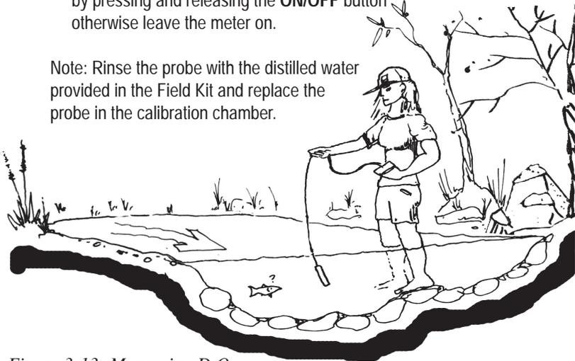
Figure 3-13: Measuring D.O.
