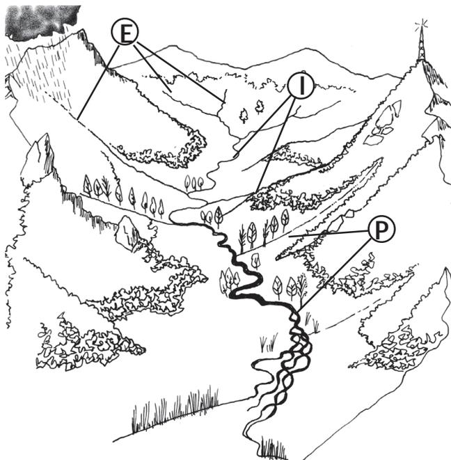
*Figure 2-10: The Stream Continuum. The top of the watershed is characterized by ephemeral headwater streams (E) with steep gradients and large substrates. These are followed by intermittent (I) and perennial (P) streams with a lower gradient and a finer substrate. If the gradient becomes shallow enough, the stream can become braided with silty substrates.(adapted from figure 1, USDA report rm-245)*
