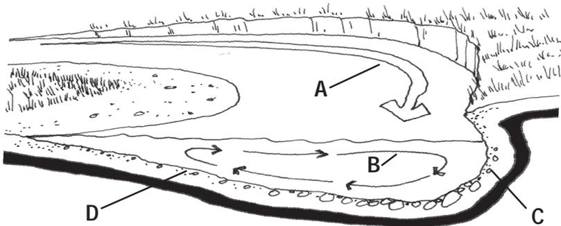
Figure 2-11: Erosion and deposition along stream curves: A) path of current around curve, B) circulatory current in water flowing around curve, C) area of erosion and D) area of deposition (from figure 28, Leopold "Water, Rivers and Creeks" 1997)
