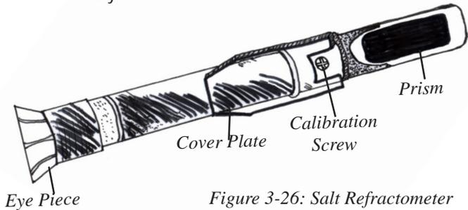
Figure 3-26: Salt Refractometer
