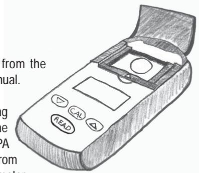
Figure 3-2: LaMotte 2020 Turbidimeter
