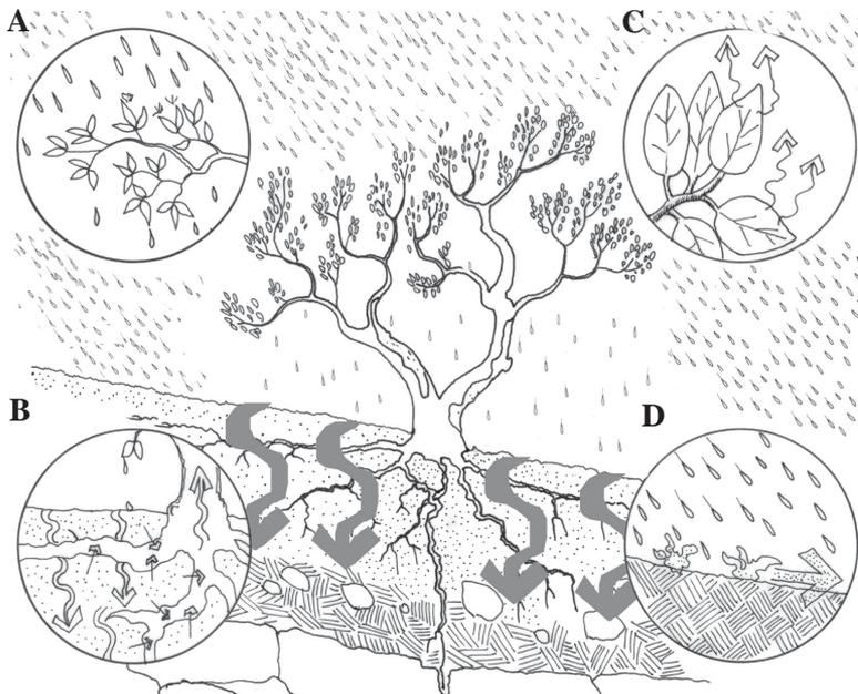
*Figure 2-4: Vegetation helps infiltration and prevents erosion by: A) intercepting the rain and slowing down water flows, B) roots break up soils creating pore space for water to infiltrate, and C) water absorbed by roots can be transpired from the leaves. D) Rain loosening exposed soils and transporting sediments into receiving waters.*
