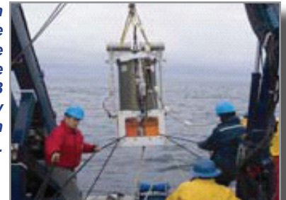
Fig. 7. Deployment of an environmental sample processor (ESP), a device used for near real-time detection of one HAB species (Monterey Bay Aquarium Research Institute).
