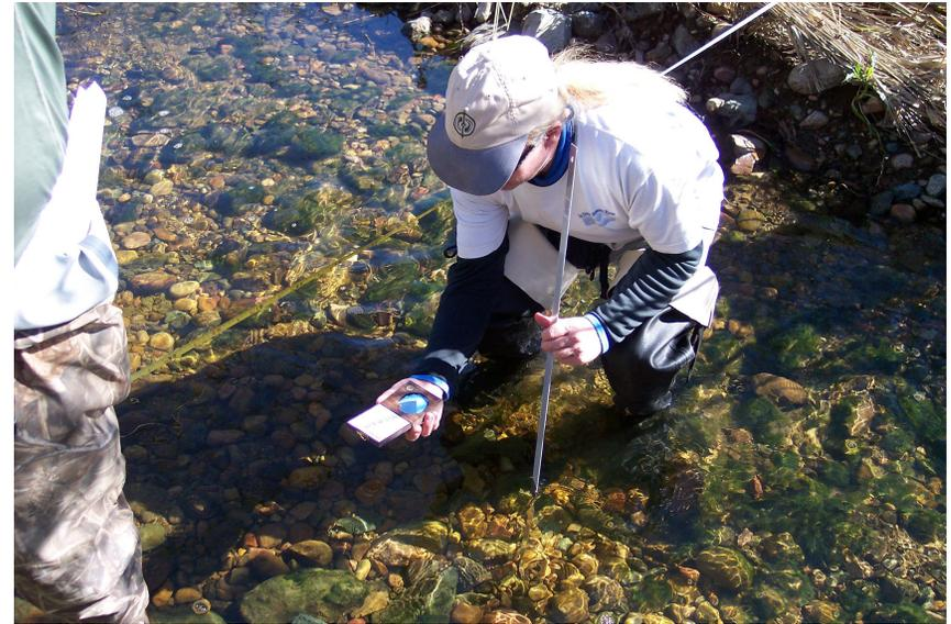
Step 1. Using a modified convex spherical densitometer, take and record four 17 point readings all taken from the center of each transect: a) facing upstream, b) facing downstream, c) facing the left bank, d) facing the right bank.
