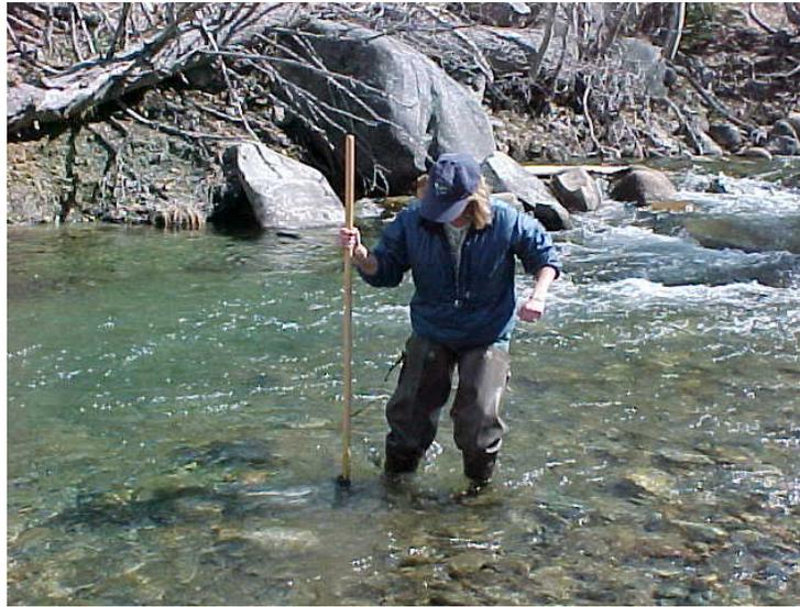
RWB -Step 5. Vigorously kick the remaining finer substrate within the quadrat with your feet while dragging the net repeatedly through the disturbed area just above the bottom. Keep moving the net all the time so that the organisms trapped in the net will not escape.
