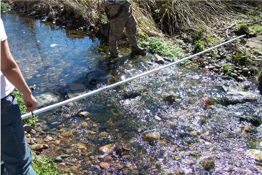
Step 3. Determine if the average wetted width is greater or less than 10 m. If average wetted width is less than 10 m use a 150 m reach length. If average wetted width  $>$  10 m then use a 250 m reach length.
