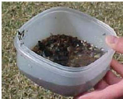
Figure 11. These processes are repeated until all organic material larger than 500 micron within the sample has been removed from the sample. Some sediment may still remain. This sample material can now be preserved.
