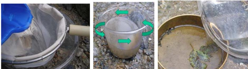
Figures 8-10. Additional water is added to remaining sample by pouring creek water through a 500 micron mesh net. The mixture is again swirled to a vortex and then poured into a 500 micron mesh sieve.
