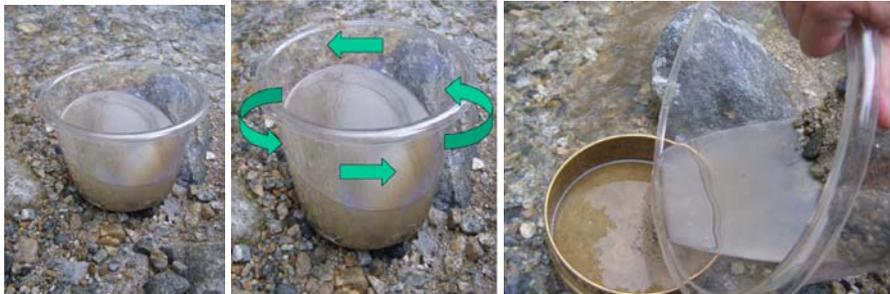
Figures 4-7. Sample and water in a bucket. Mixture is swirled to a vortex and then poured into a 500 micron mesh sieve.
