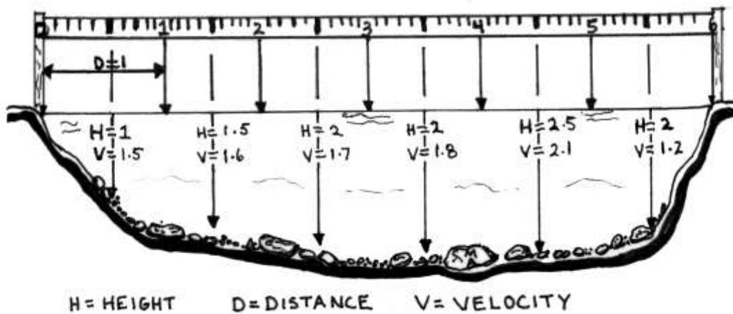
**Figure 6: diagram of areas and associated velocity for individual cells**
