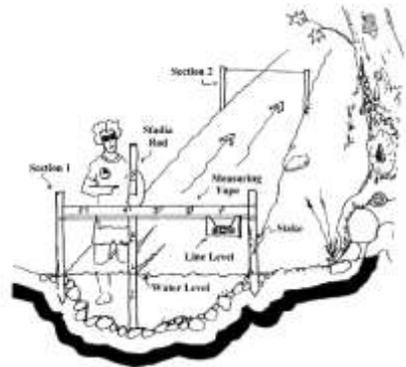
6. Add up the depths on the Stream Flow Field Sheet. This is the cross sectional area for that section of the stream.
