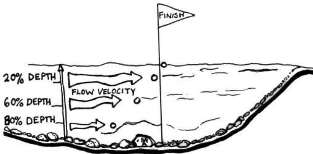
**Figure 5. Variation in velocity with depth within stream**
