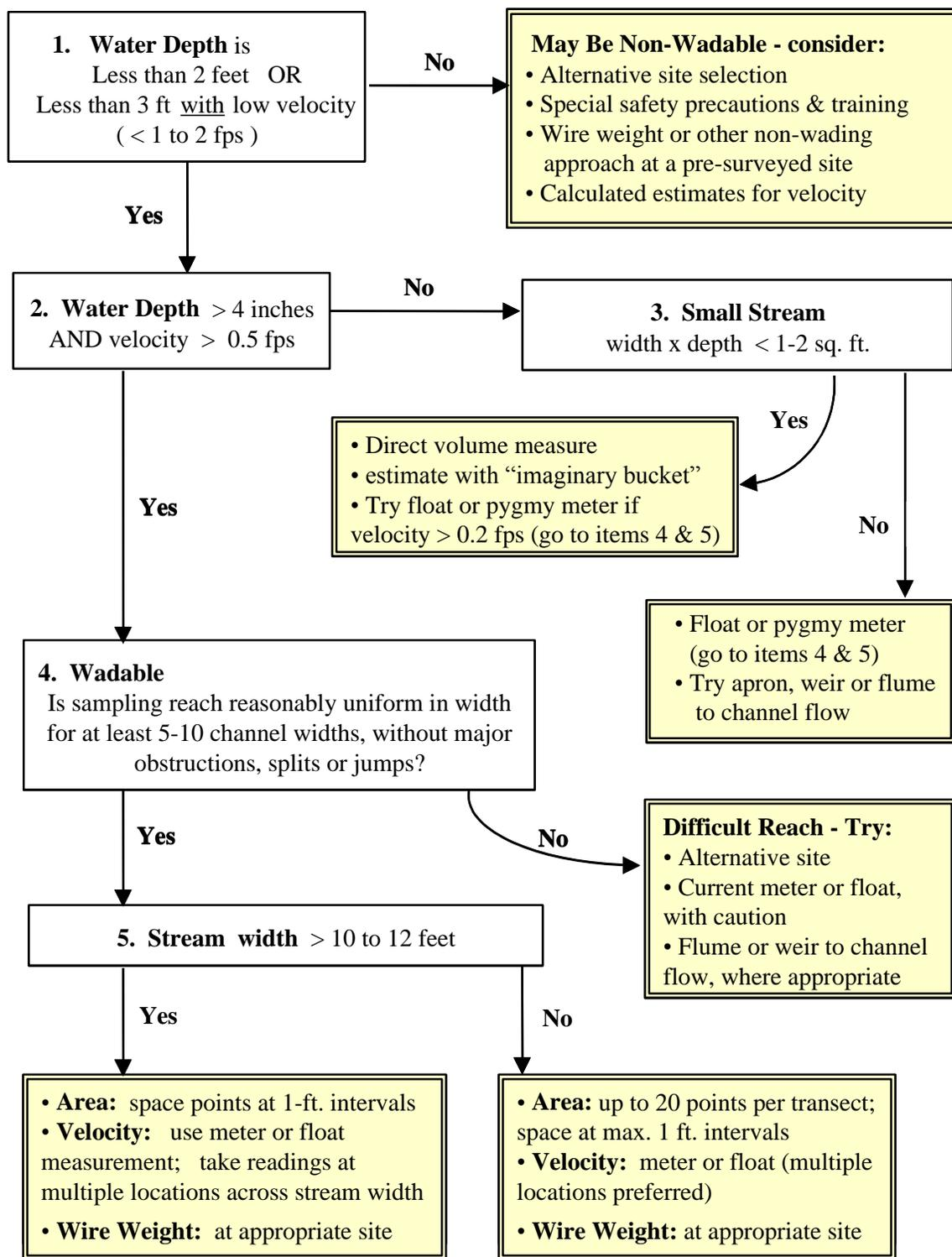
Figure 1. Decision flow chart for selection of flow measurement method
