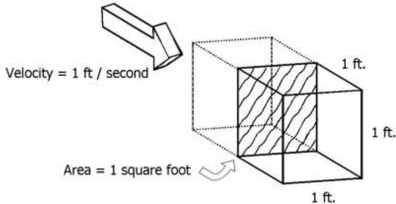
**Figure 2. Principles of velocity-area flow measurement**
