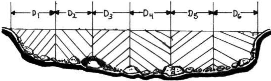
**Figure 3: schematic channel cross section with imaginary rectangular "cells"**
