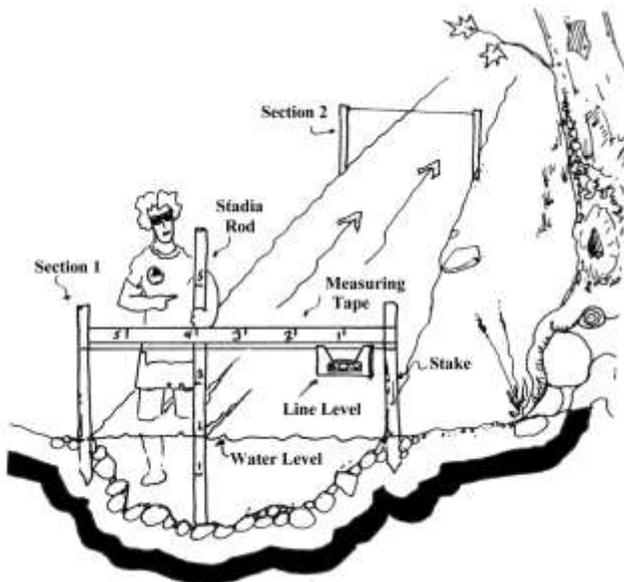
**Figure 4. Taglines marking ends of stream segment used for float measurement**
