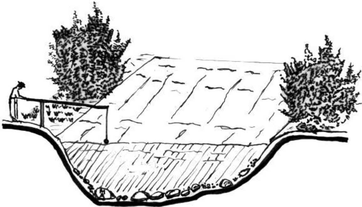
**Figure 8 wire weight gaging from fixed vantage point (after Napa RCD, 1998)**
