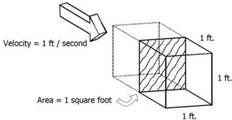
**Figure 2. Principles of velocity-area flow measurement**
