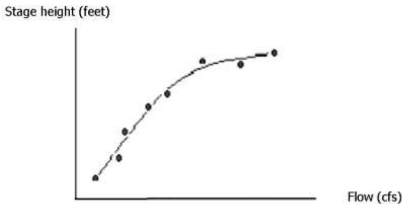
**Figure 7: simplified rating curve**
