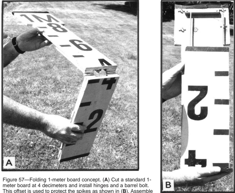
Figure 57—Folding 1-meter board concept. (A) Cut a standard 1-meter board at 4 decimeters and install hinges and a barrel bolt. This offset is used to protect the spikes as shown in (B). Assemble the board before painting and application of decimeter marks to assure correct measurements.
