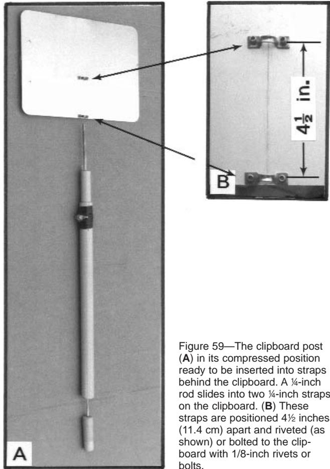
Figure 59—The clipboard post (A) in its compressed position ready to be inserted into straps behind the clipboard. A 1/4-inch rod slides into two 1/4-inch straps on the clipboard. (B) These straps are positioned 4 1/2 inches (11.4 cm) apart and riveted (as shown) or bolted to the clipboard with 1/8-inch rivets or bolts.
