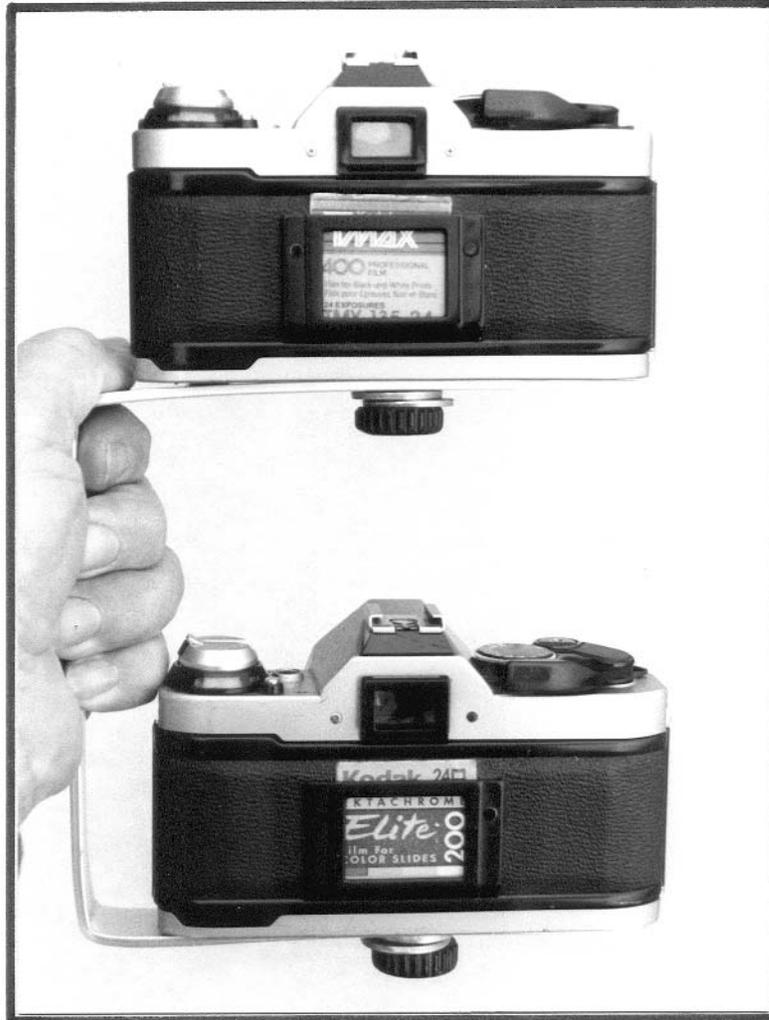
Figure 64—Double camera bracket for use when photographing in both color and black and white. The bracket is made from 1-inch by  $\frac{1}{8}$ -inch aluminum bar-stock with holes drilled to mount the cameras. Identical cameras are recommended to simplify camera adjustments. Figures 65 and 66 illustrate construction details.
