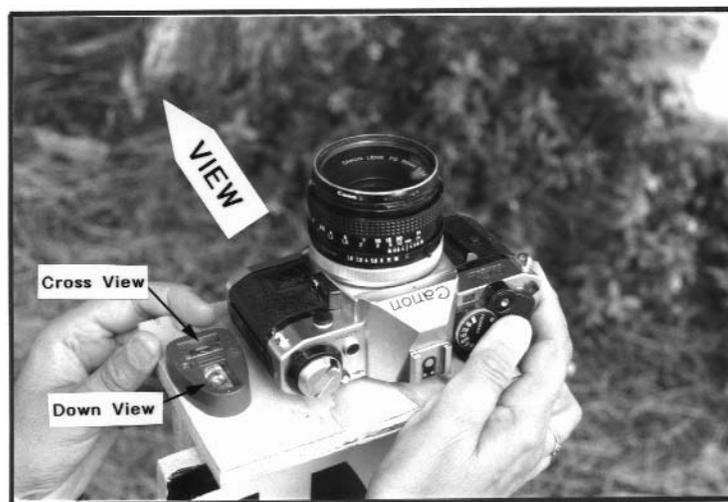
Figure 63—The camera leveling board is used to take repeat photographs of the tree canopy with some consistency. Place the leveling board on top of the meter board for consistent height above the ground. Place the meter board at right angles to the photo view. Move the meter board sideways to center the cross-view bubble, then tilt the level board to center the down-view bubble, move your head back, and photograph.
