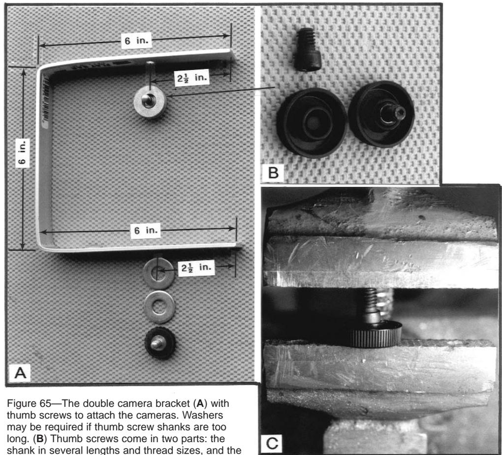
Figure 65—The double camera bracket (A) with thumb screws to attach the cameras. Washers may be required if thumb screw shanks are too long. (B) Thumb screws come in two parts: the shank in several lengths and thread sizes, and the head. The head must be forced onto the shank by using a vise (C). A shank diameter of 1/4 inch, length of 3/8 inch, and 20 threads per inch fits many cameras.
