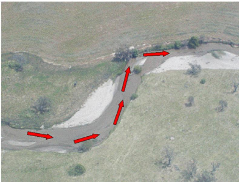
Fig. 2 - The red arrows show the line of highest velocity and depth known as the **thalweg**. This swings from side to side causing erosion at the apex of bends and deposition on point bars on the inside of bends. Picture by Dr. Tim Stott
