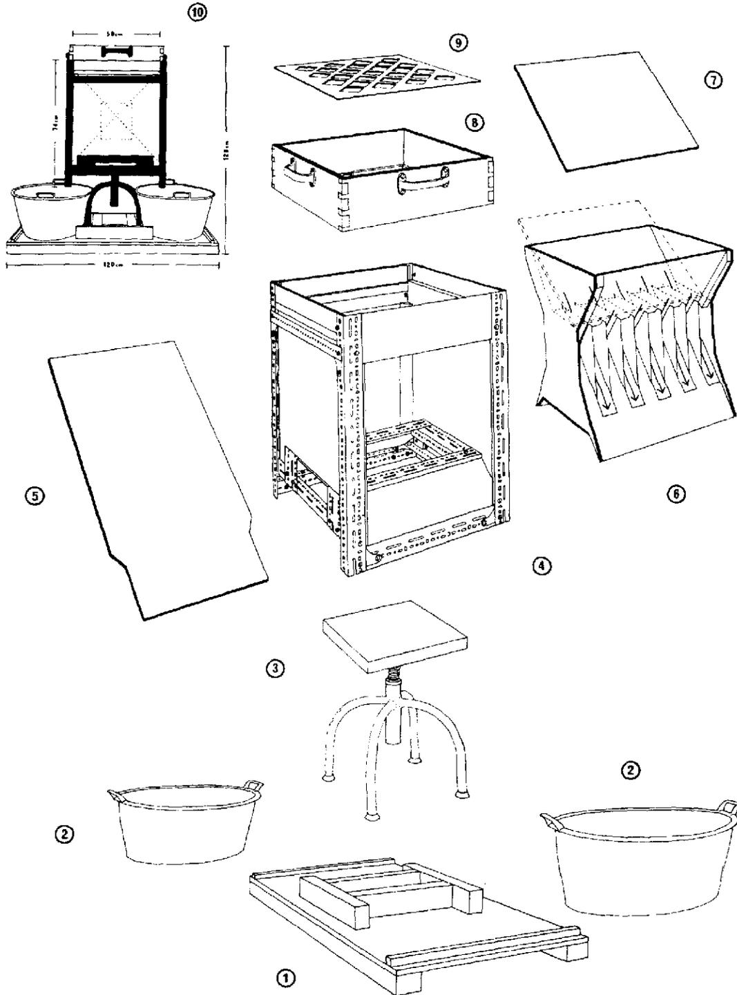
Fig. 2.10: A sieving and splitting device: (1) basal plate, (2) catch bins, (3) rockable, springy stand, (4) central frame, (5) deflecting board, (6) riffle splitter, (7) splitter board, (8) screen frame, (9) screen, (10) assembled device with general measurements (Reprinted from Ibbeken (1974), by permission of the Society of Sedimentary Geology).
