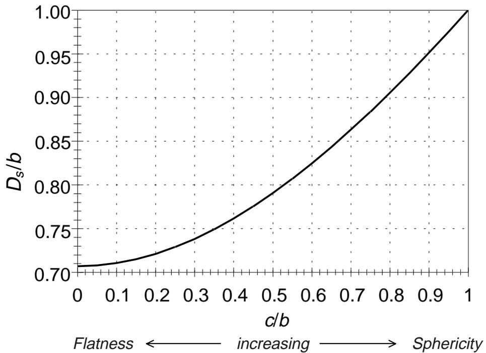
Fig. 2.4: Ratio of square-hole sieve opening  $D_s$  to measured  $b$ -axis size as a function of particle flatness, i.e., the ratio of  $c/b$  (Redrawn from Church et al. 1987; by permission of John Wiley and Sons, Ltd.).
