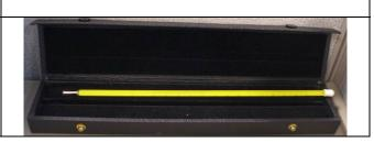
Certified Thermometer (Partial Immersion) Traceable to NIST and DKD/PTB, with calibration certificate and protective foam. Range: -1 to 61°C, 0.1 Div., 76mm www.hbinstrument.com (800)4-test-lab Catalog No. 20528 14ct.
